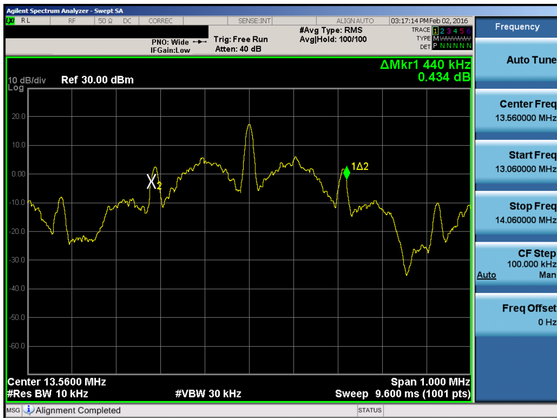
Figure 8-2. 20dB Bandwidth Plot
