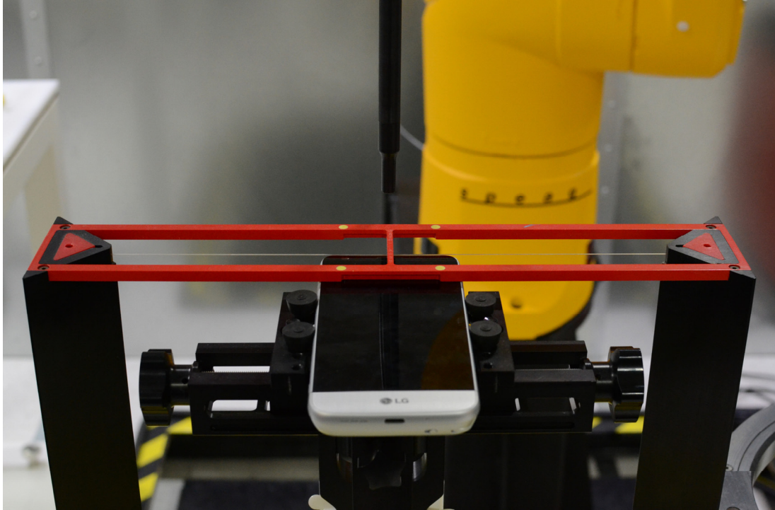
Figure 18-3 Ear Reference Point HAC Phantom Alignment – Camera Module Accessory
