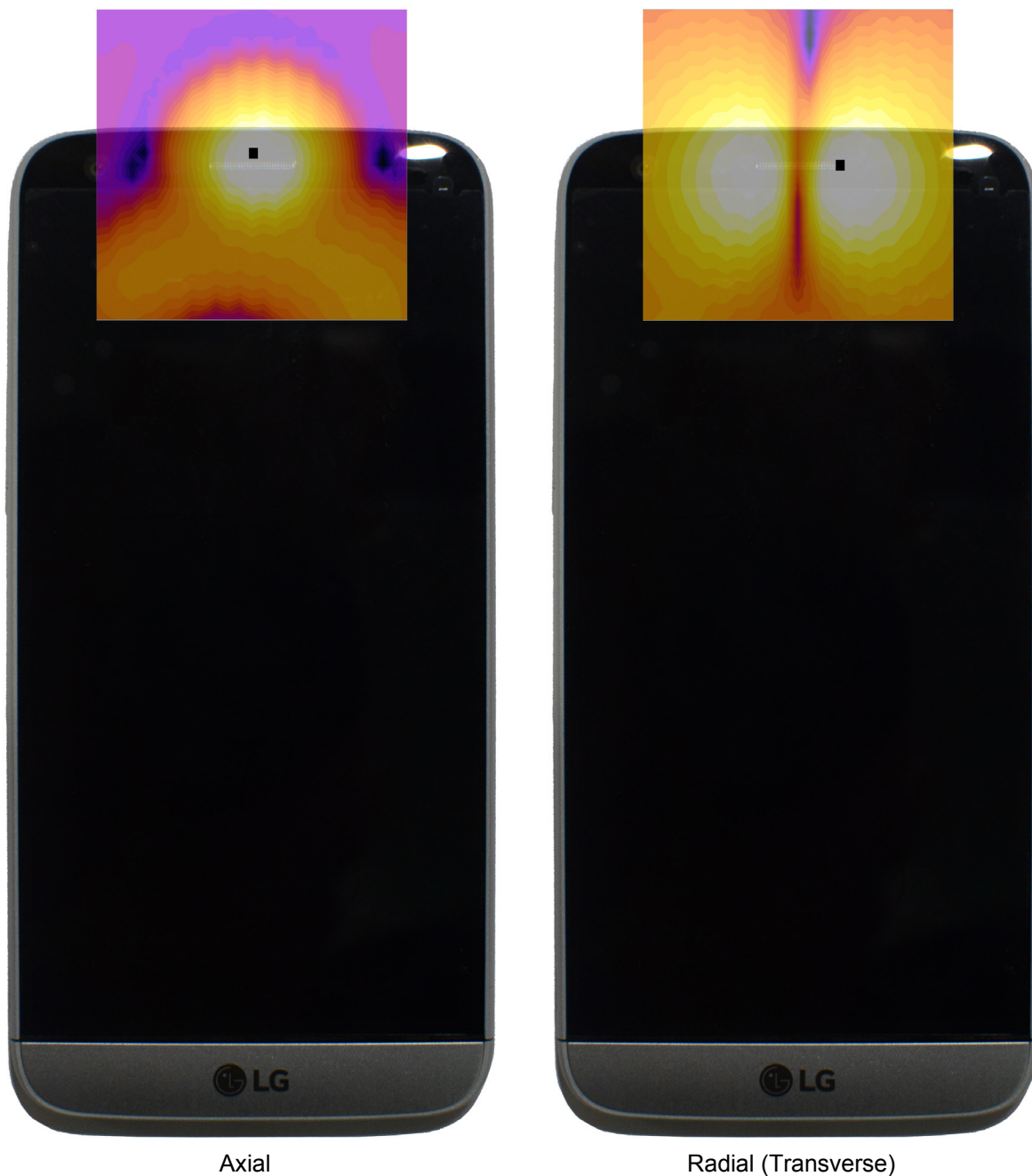
Figure 15-5 T-Coil Scan Overlay Magnetic Field Distributions
