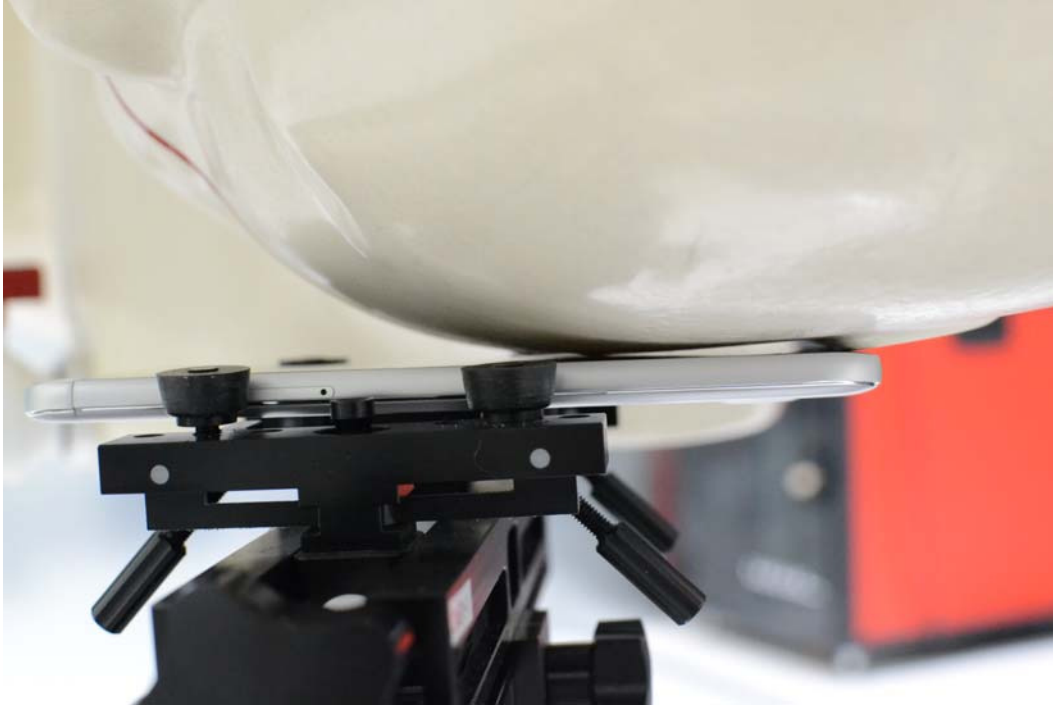
SAR Test Setup Photo 5: Left Cheek
