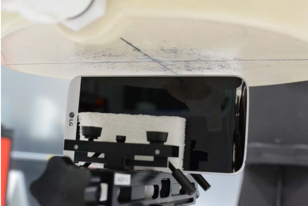
SAR Test Setup Photo 19: Left at 1.0 cm
