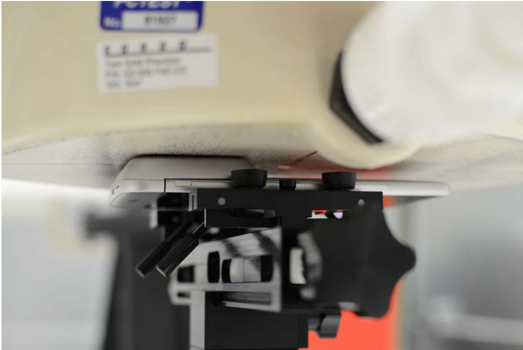
SAR Test Setup Photo 11: Back at 0.0 cm Camera Module Accessory
