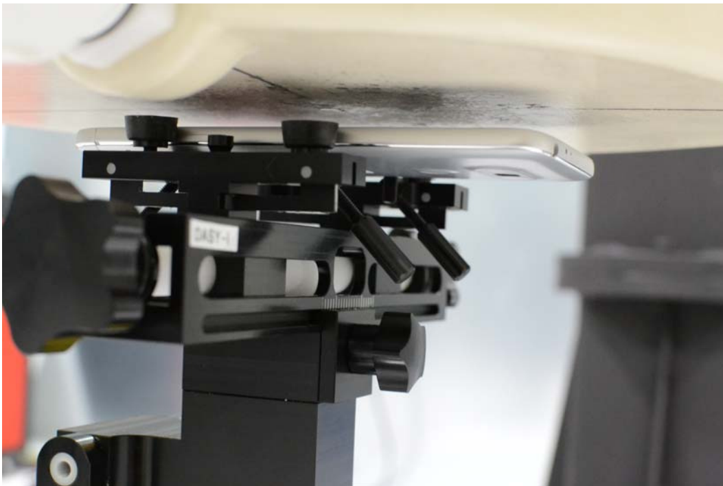
SAR Test Setup Photo 12: Front at 1.0 cm
