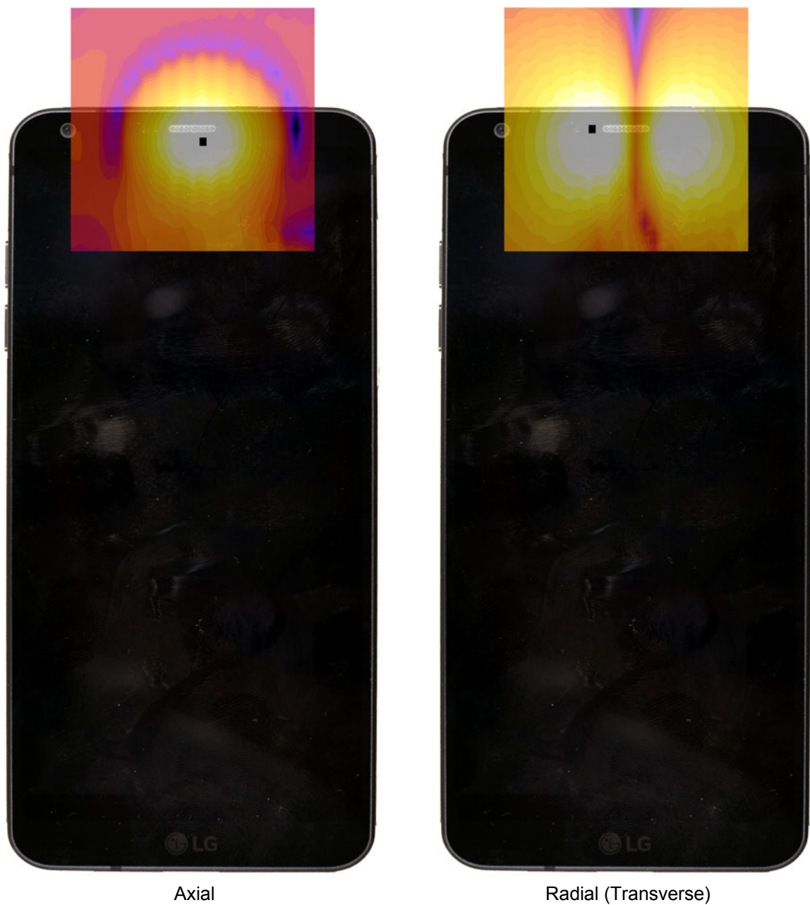
Axial Radial (Transverse) Figure 14-3 T-Coil Scan Overlay Magnetic Field Distributions
