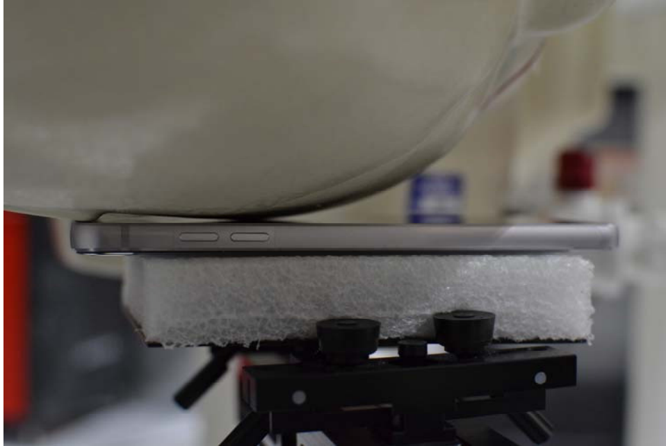
SAR Test Setup Photo 1: Right Cheek
