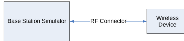
Figure 9-3 Power Measurement Setup
