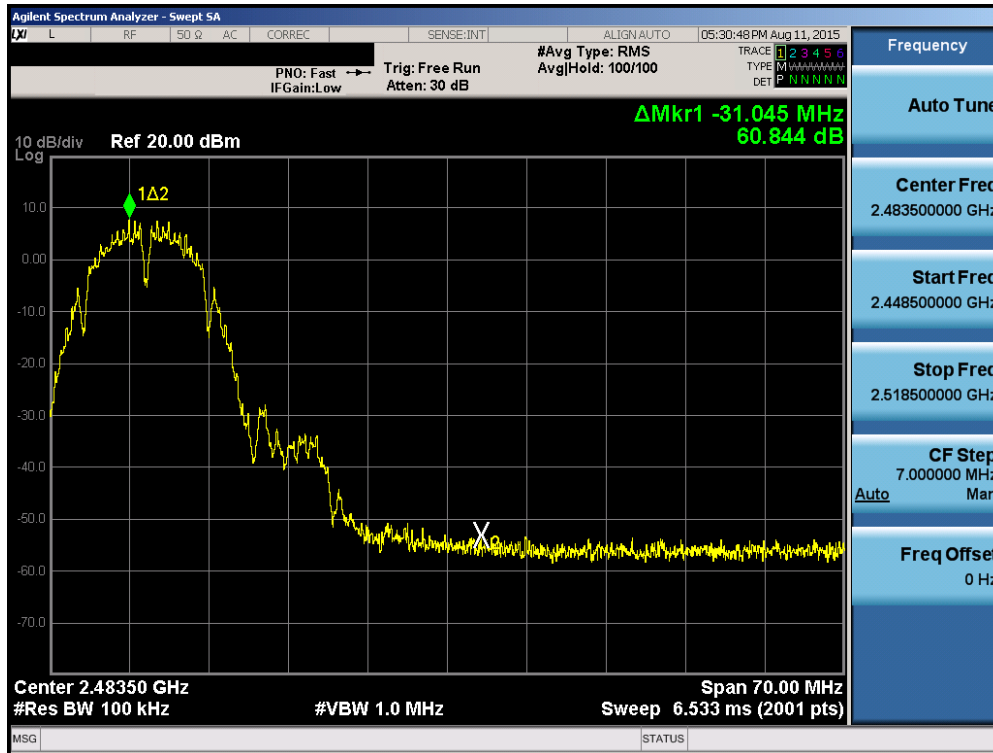
Plot 6-21. Band Edge Plot (802.11b – Ch. 10)
