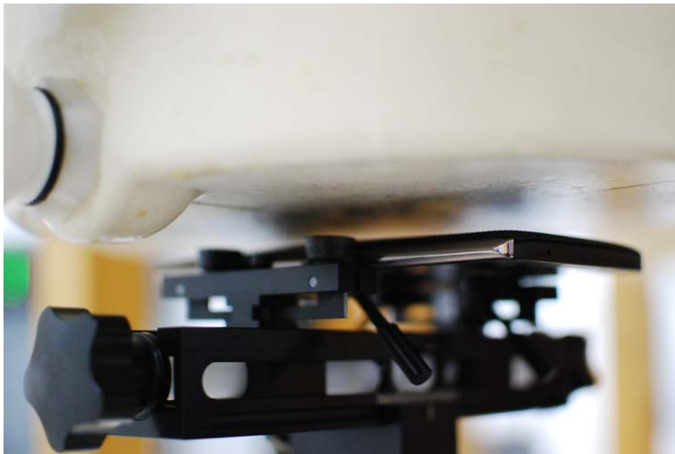
SAR Test Setup Photo 8: Back Side, Wireless Charging Cover at 10 mm
