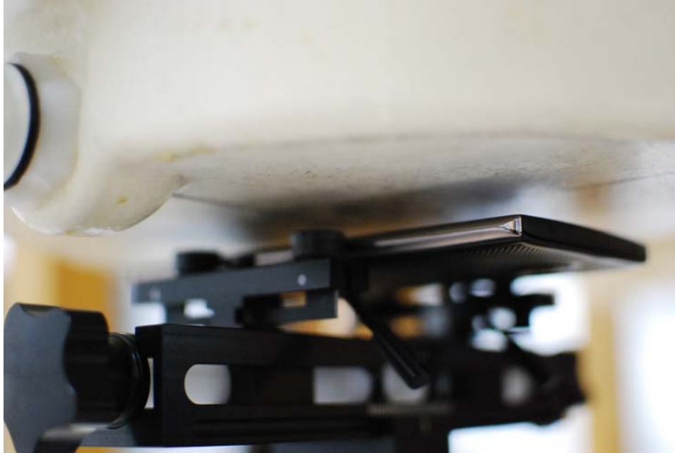
SAR Test Setup Photo 11: Front Side, Standard Cover at 10 mm
