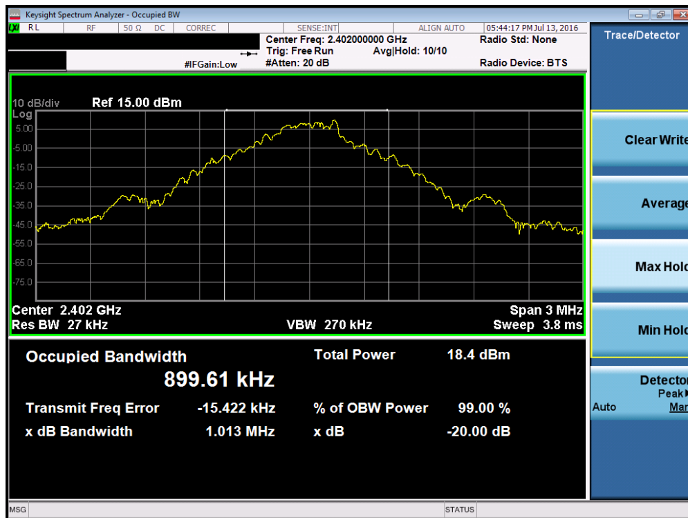
Plot 7-1. 20dB Bandwidth Plot (Bluetooth, 1Mbps – Ch. 0)
