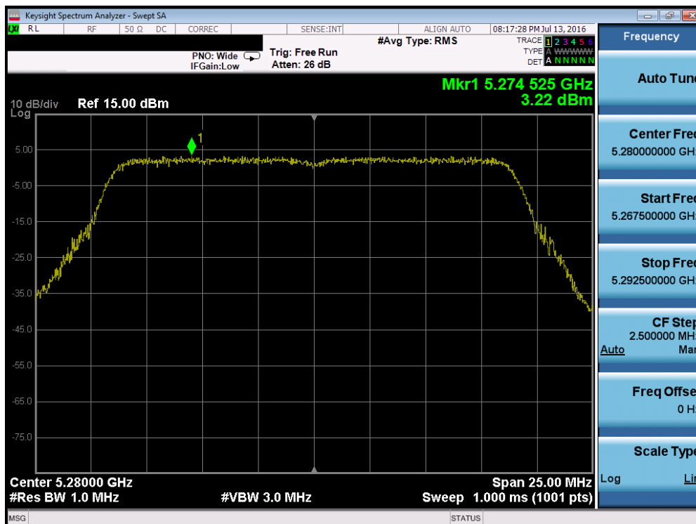
Plot 7-128. Power Spectral Density Plot (20MHz BW 802.11n (UNII Band 2A) – Ch. 56)
