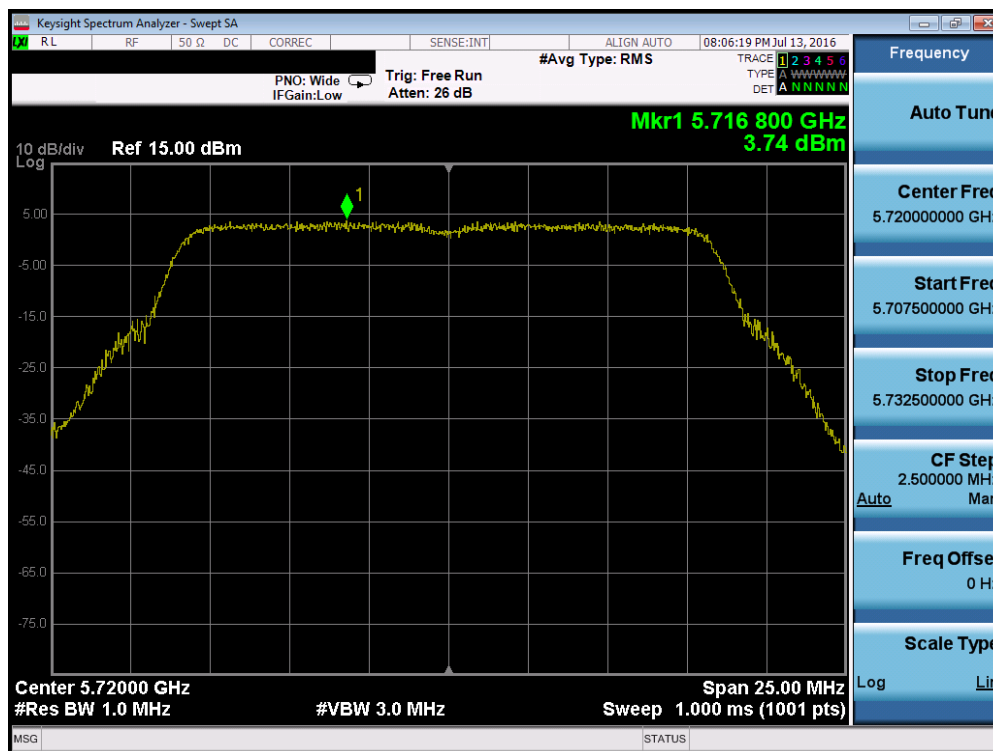
Plot 7-135. Power Spectral Density Plot (802.11a (UNII Band 2C) – Ch. 144)
