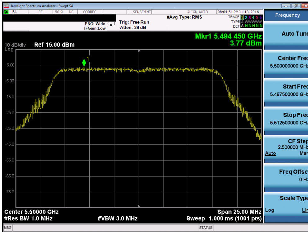
Plot 7-133. Power Spectral Density Plot (802.11a (UNII Band 2C) – Ch. 100)
