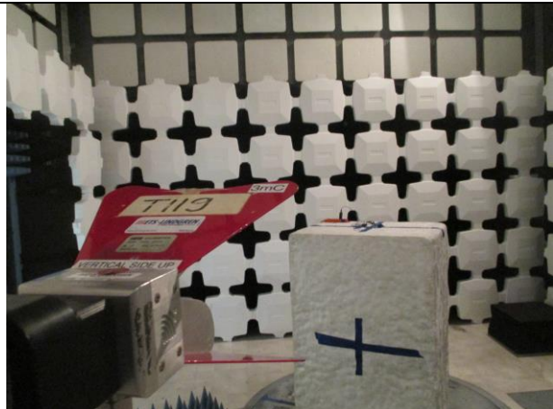
RADIATED BACK PHOTO (ABOVE 1 GHz)
