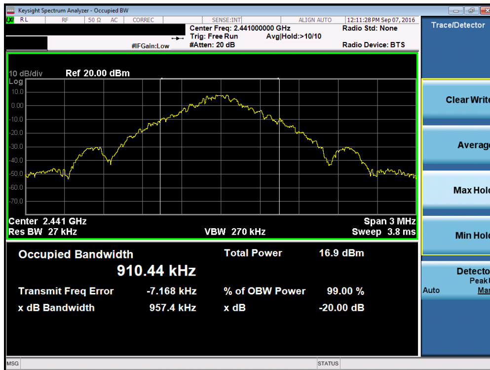
Plot 7-2. 20dB Bandwidth Plot (Bluetooth, 1Mbps – Ch. 39)
