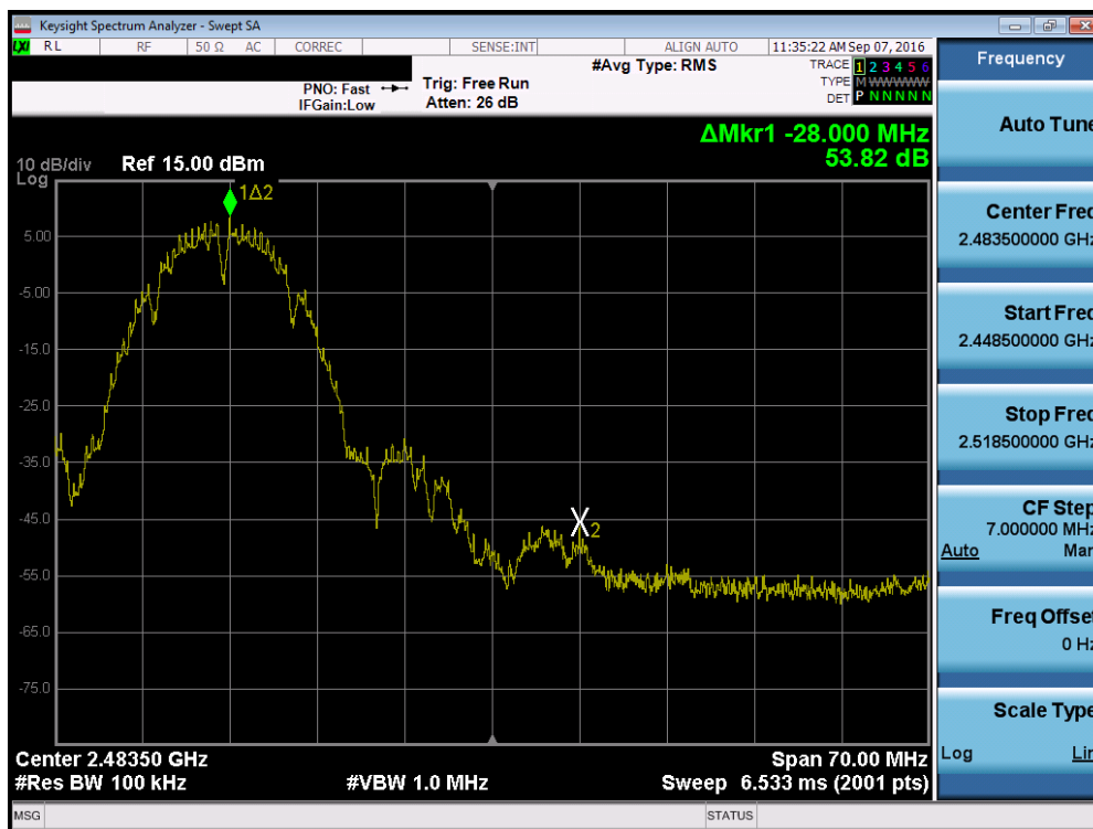
Plot 7-23. Band Edge Plot (802.11b – Ch. 11)
