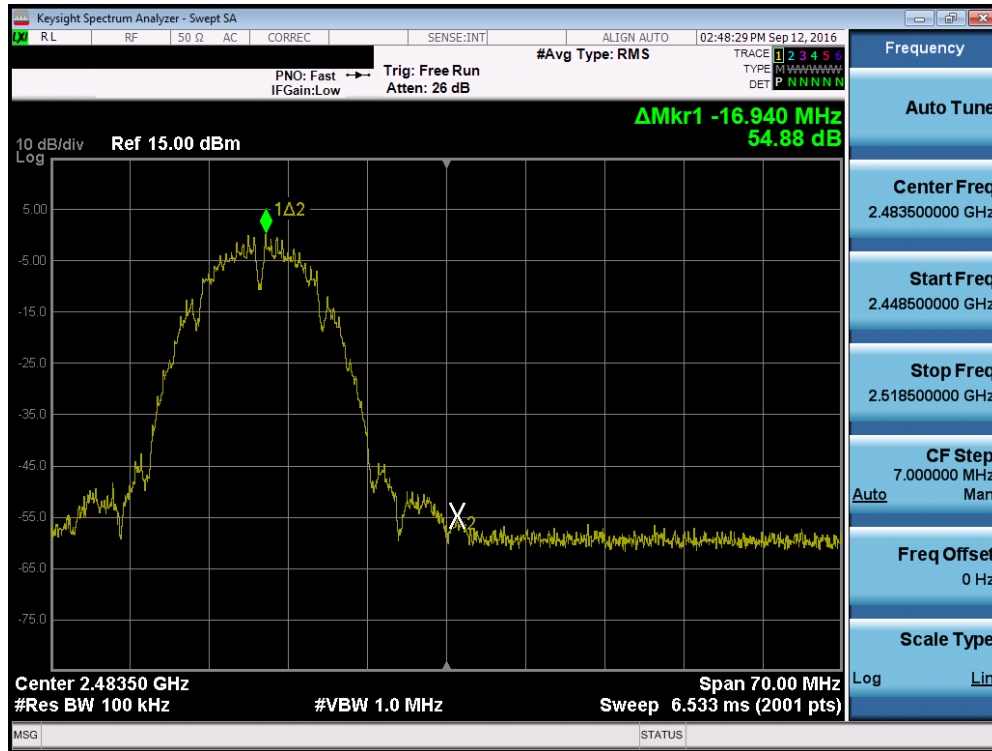
Plot 7-24. Band Edge Plot (802.11b – Ch. 12)
