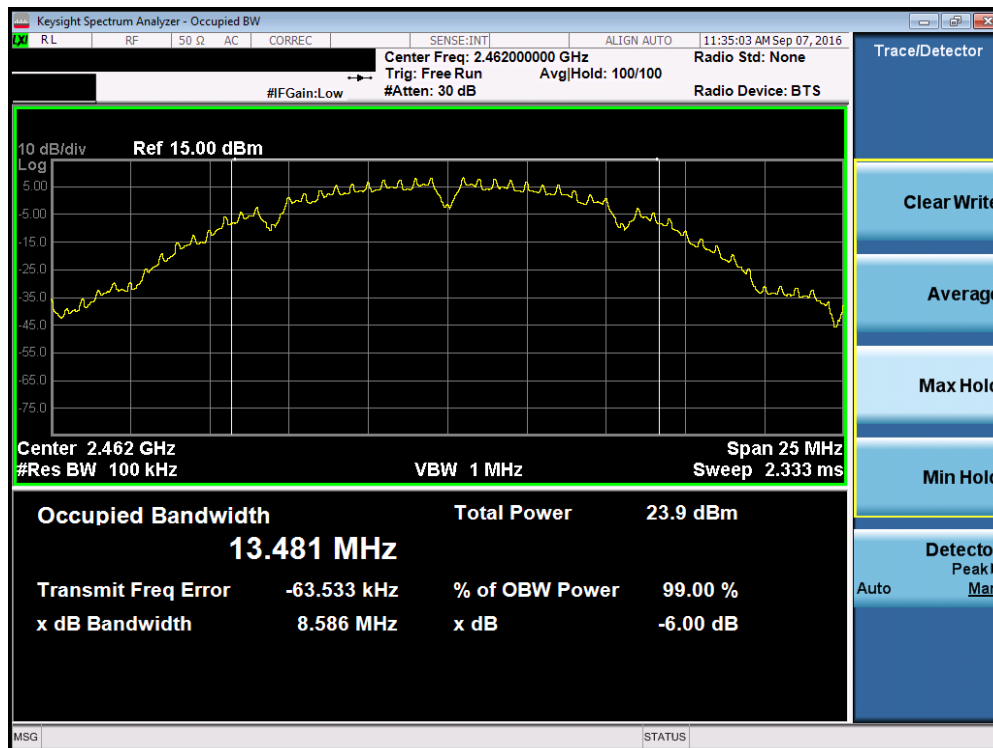
Plot 7-3. 6dB Bandwidth Plot (802.11b – Ch. 11)
