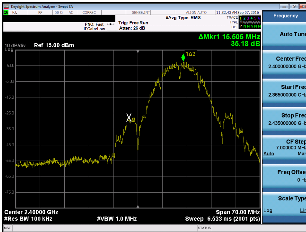
Plot 7-22. Band Edge Plot (802.11b – Ch. 1)
