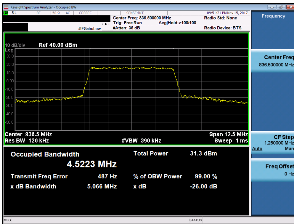
Plot 7-14. Occupied Bandwidth Plot (Band 5 – 5.0MHz QPSK - Full RB Configuration)
