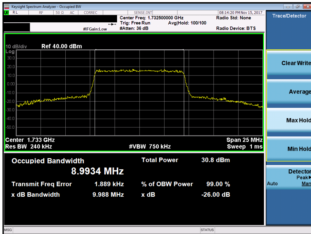
Plot 7-24. Occupied Bandwidth Plot (Band 4 - 10.0MHz 16-QAM - Full RB Configuration)
