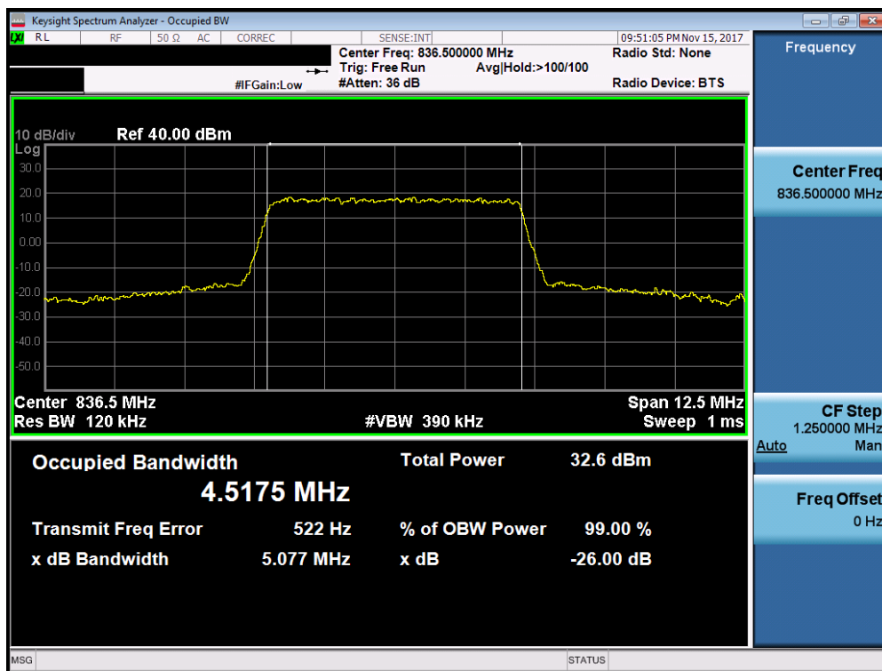
Plot 7-13. Occupied Bandwidth Plot (Band 5 – 5.0MHz QPSK - Full RB Configuration)
