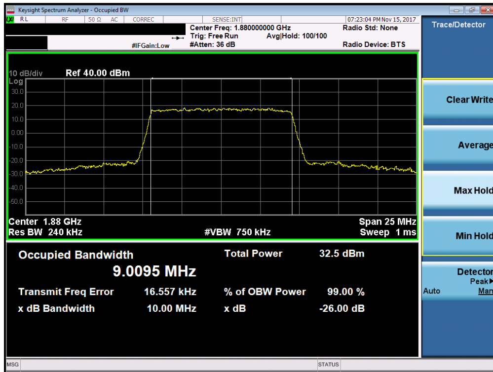
Plot 7-35. Occupied Bandwidth Plot (Band 2 - 10.0MHz QPSK - Full RB Configuration)
