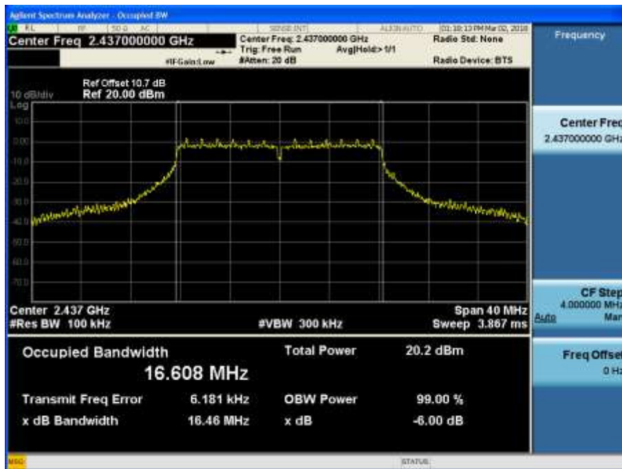
6dB Bandwidth plot (802.11g-CH 6)
