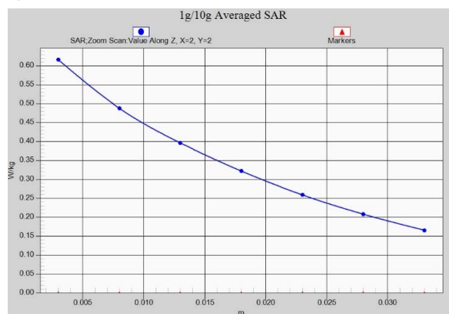
Fig.A.1- 9 Z-Scan at power reference point (W850)
