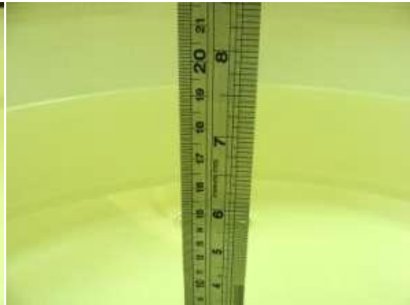
Photo of Liquid Height for Body SAR
