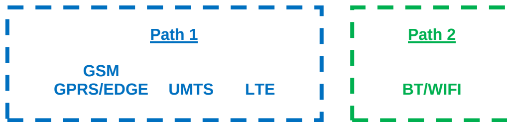
Figure 1-1 Simultaneous Transmission Paths
