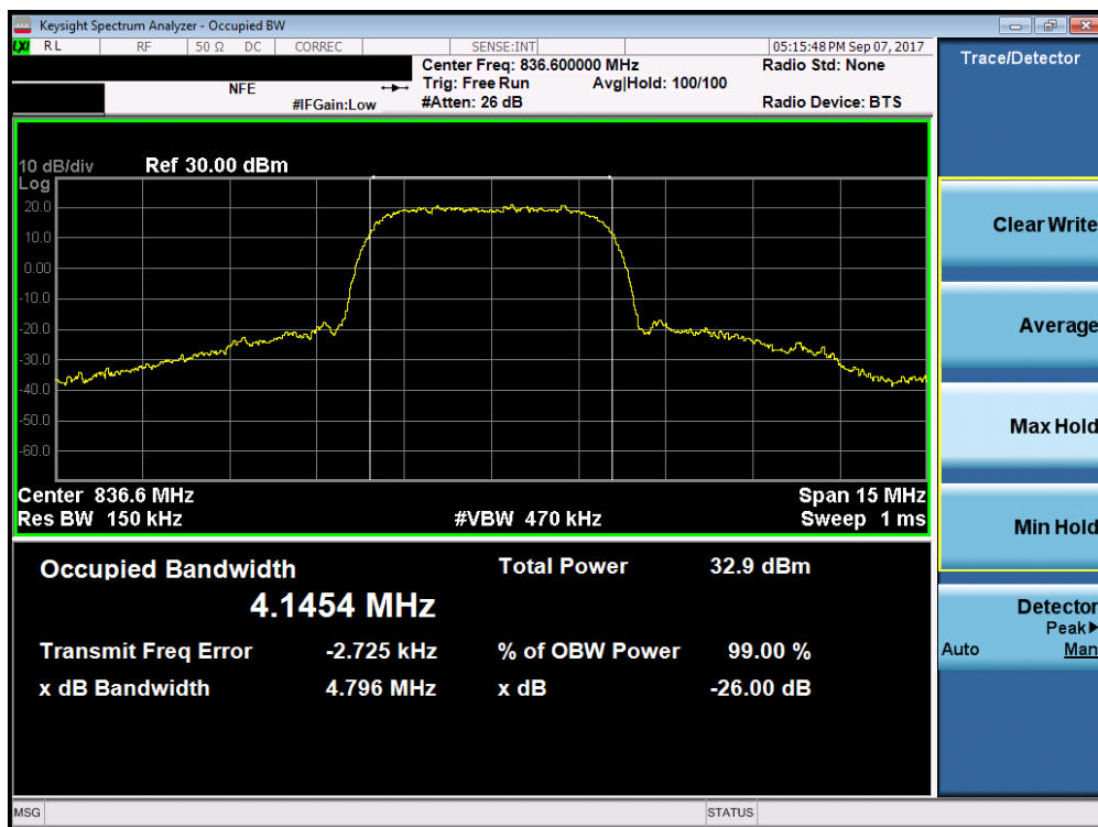
Plot 7-5. Occupied Bandwidth Plot (Cellular WCDMA Mode)
