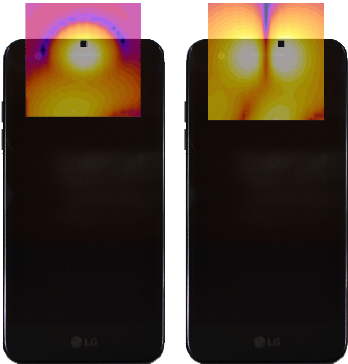
Figure 13-3 T-Coil Scan Overlay Magnetic Field Distributions
