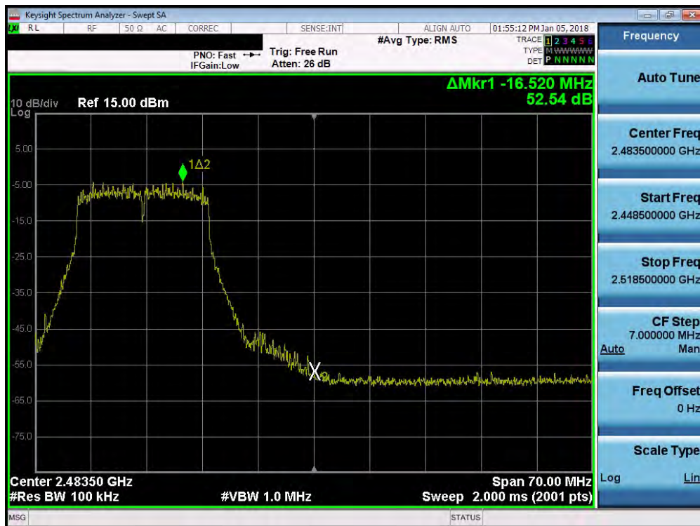
Plot 7-22. Band Edge Plot (802.11g – Ch. 11)
