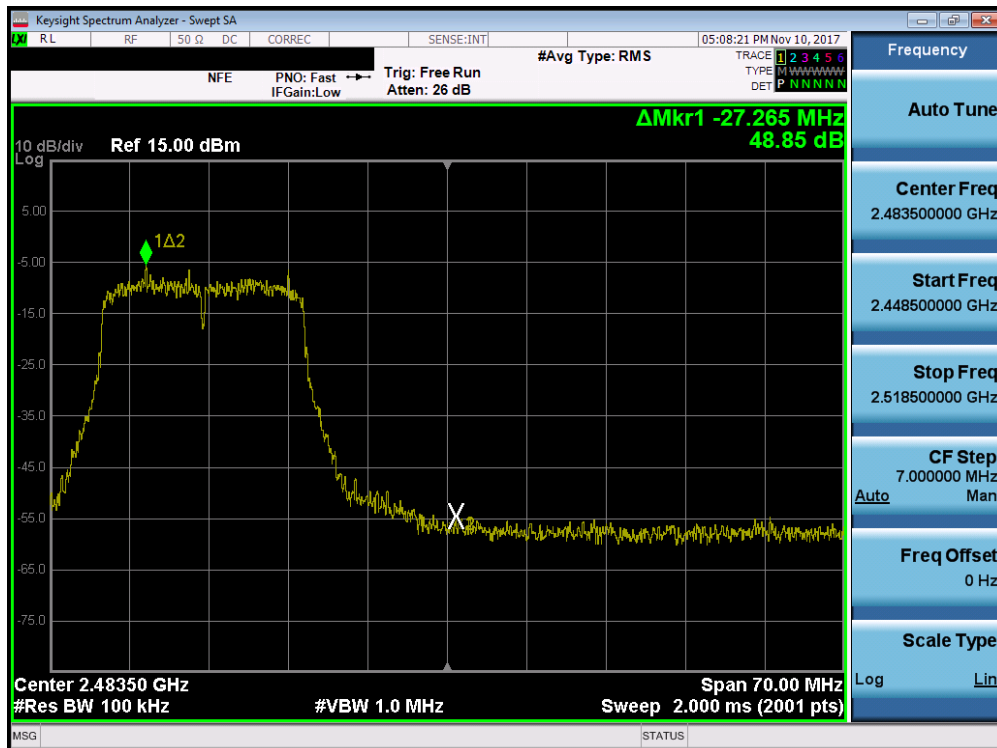
Plot 7-24. Band Edge Plot (802.11n (2.4GHz) – Ch. 11)
