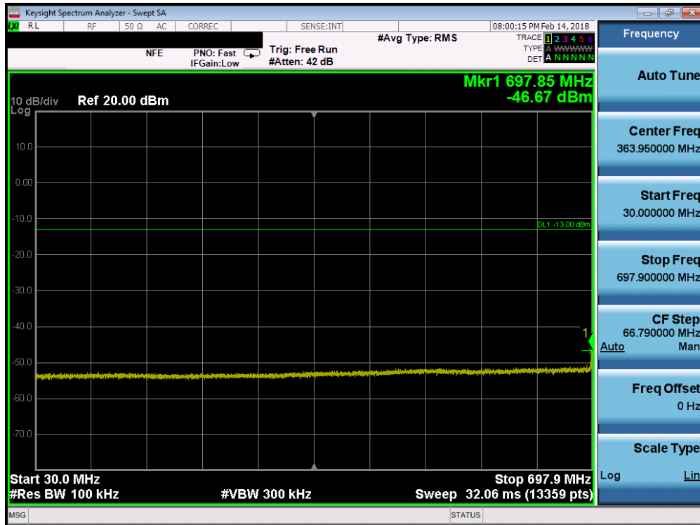
Plot 7-58. Conducted Spurious Plot (Band 12 - 10.0MHz QPSK - RB Size 1, RB Offset 0 - Low Channel)
