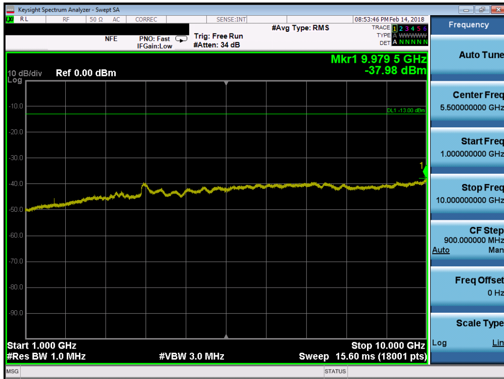
Plot 7-69. Conducted Spurious Plot (Band 5 - 10.0MHz QPSK - RB Size 1, RB Offset 0 - Low Channel)
