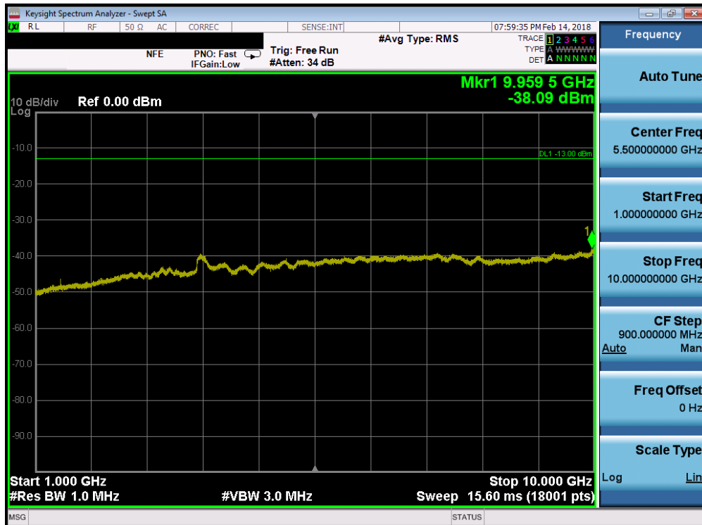
Plot 7-63. Conducted Spurious Plot (Band 12 - 10.0MHz QPSK - RB Size 1, RB Offset 0 - Mid Channel)
