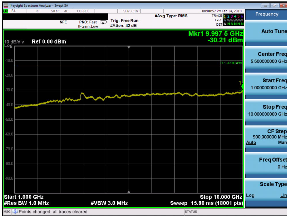
Plot 7-60. Conducted Spurious Plot (Band 12 - 10.0MHz QPSK - RB Size 1, RB Offset 0 - Low Channel)
