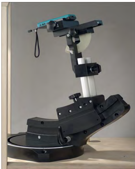
F-2. Device Holder for Transmitters
