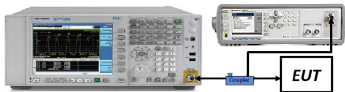
Figure 7-4. Test Instrument & Measurement Setup
