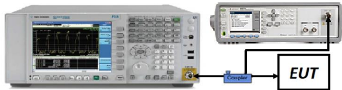
Figure 7-2. Test Instrument & Measurement Setup
