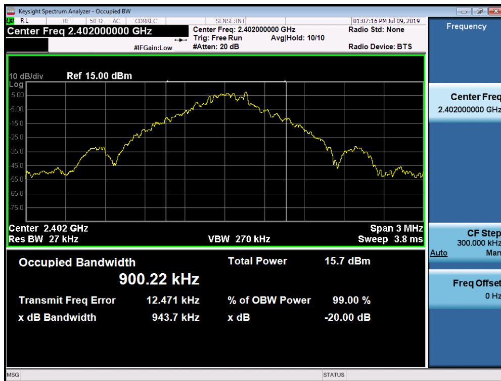
Plot 7-1. 20dB Bandwidth Plot (Bluetooth, 1Mbps – Ch. 0)
