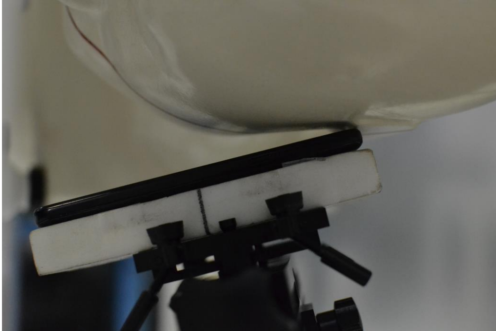
SAR Test Setup Photo 4 – Left Tilt
