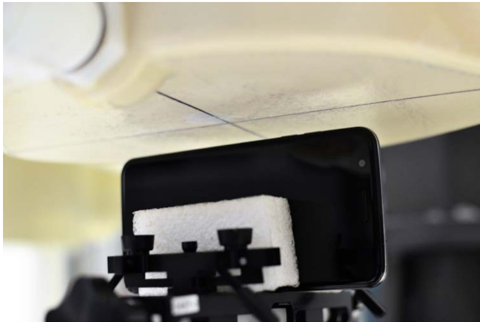
SAR Test Setup Photo 10: Left at 1.0 cm
