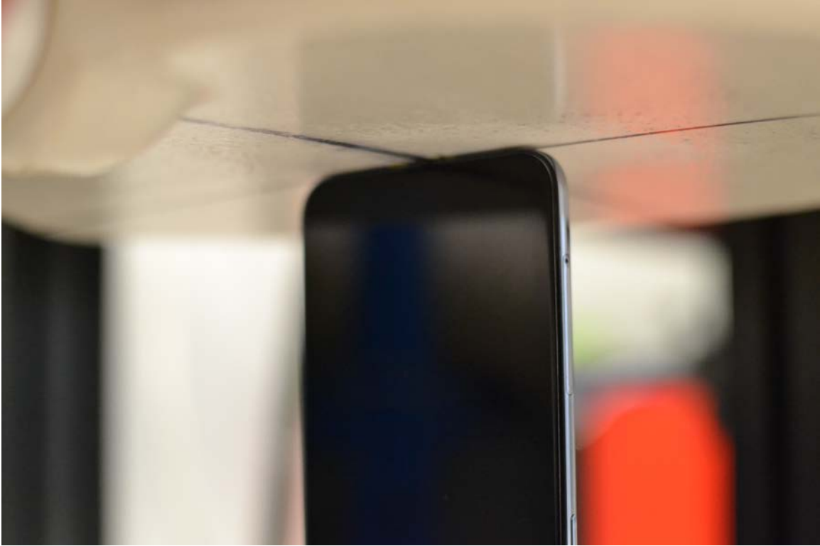
SAR Test Setup Photo 15 – Bottom Edge at 0.0cm
