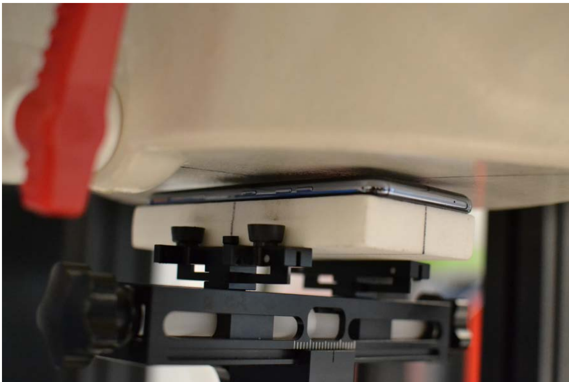
SAR Test Setup Photo 6 – Back Side at 0.3cm
