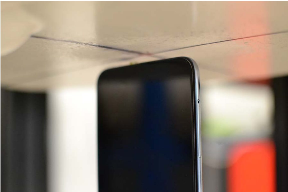
SAR Test Setup Photo 14 – Bottom Edge at 0.4cm
