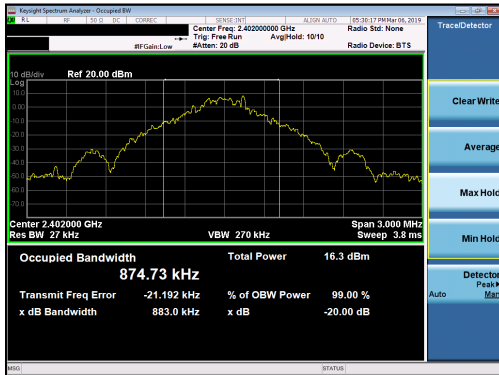
Plot 7-1. 20dB Bandwidth Plot (Bluetooth, 1Mbps – Ch. 0)
