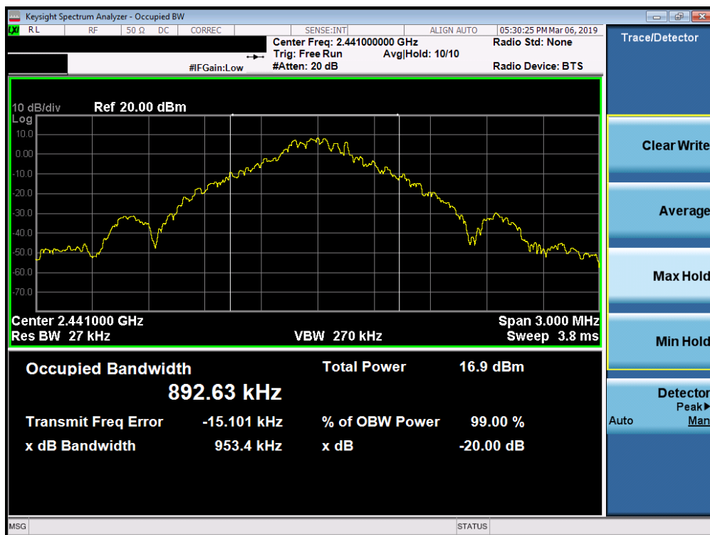
Plot 7-2. 20dB Bandwidth Plot (Bluetooth, 1Mbps – Ch. 39)
