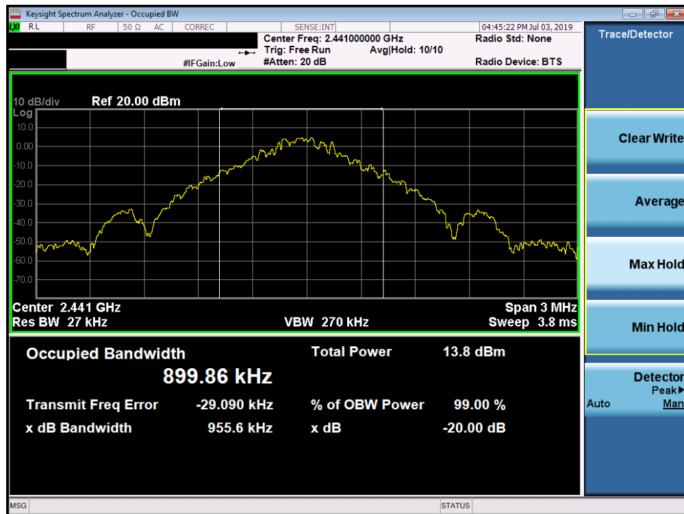
Plot 7-2. 20dB Bandwidth Plot (Bluetooth, 1Mbps – Ch. 39)
