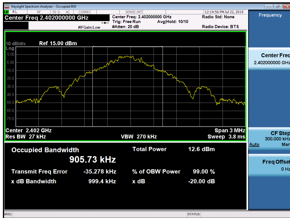
Plot 7-1. 20dB Bandwidth Plot (Bluetooth, 1Mbps – Ch. 0)
