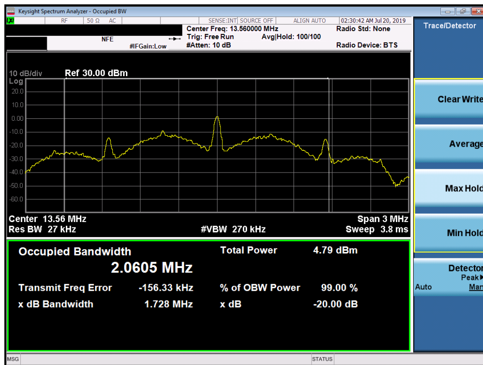
Figure 7-2. Occupied Bandwidth Plot
