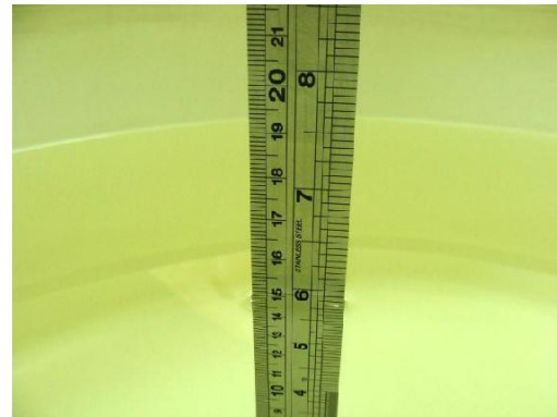
Fig 6.11 Photo of Liquid Height for Body SAR
