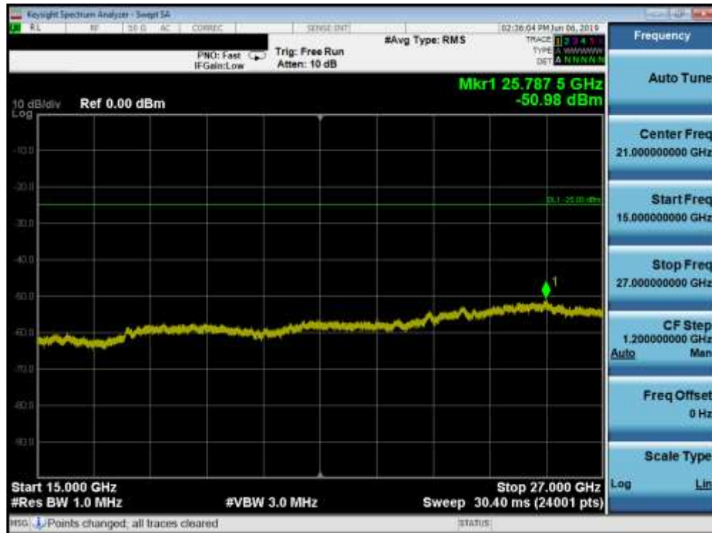
Plot 7-100. Conducted Spurious Plot (Band 7 - 20.0MHz QPSK - RB Size 1, RB Offset 0 - High Channel)
