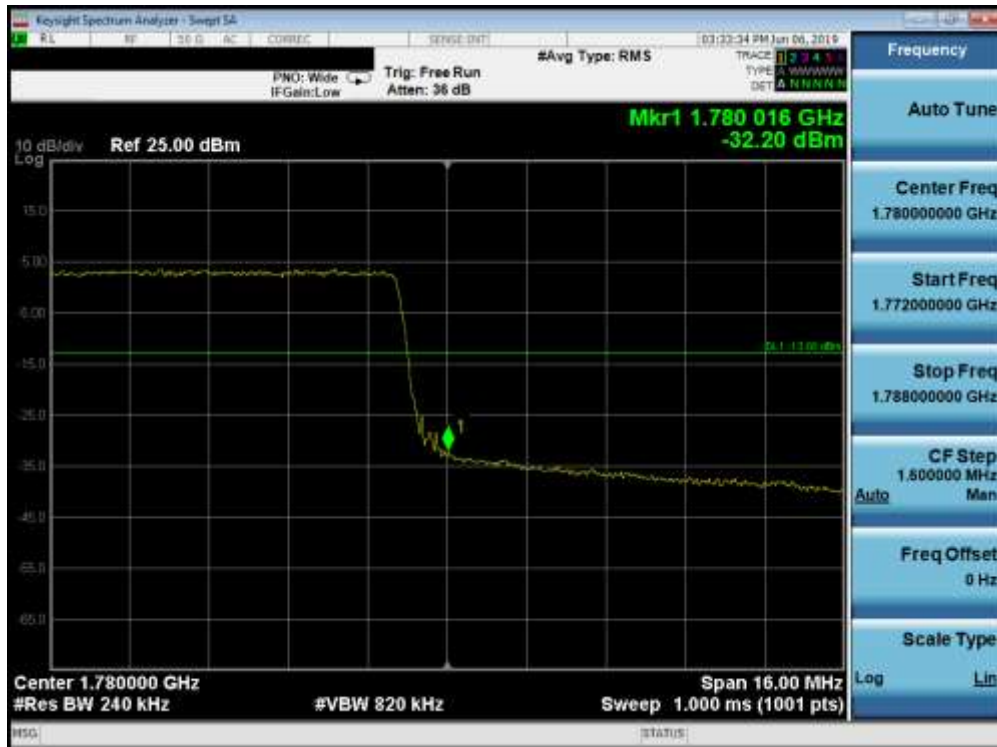
Plot 7-161. Upper Band Edge Plot (Band 66 - 20.0MHz QPSK - Full RB Configuration)
