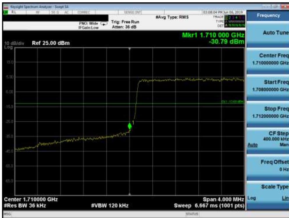
Plot 7-133. Lower Band Edge Plot (Band 66/4 - 3.0MHz QPSK - Full RB Configuration)
