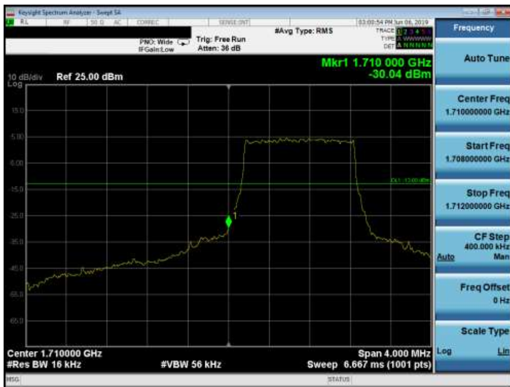
Plot 7-127. Lower Band Edge Plot (Band 66/4 - 1.4MHz QPSK - Full RB Configuration)
