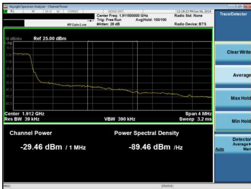
Plot 7-166. Upper Extended Band Edge Plot (Band 2 - 1.4MHz QPSK - Full RB Configuration)
