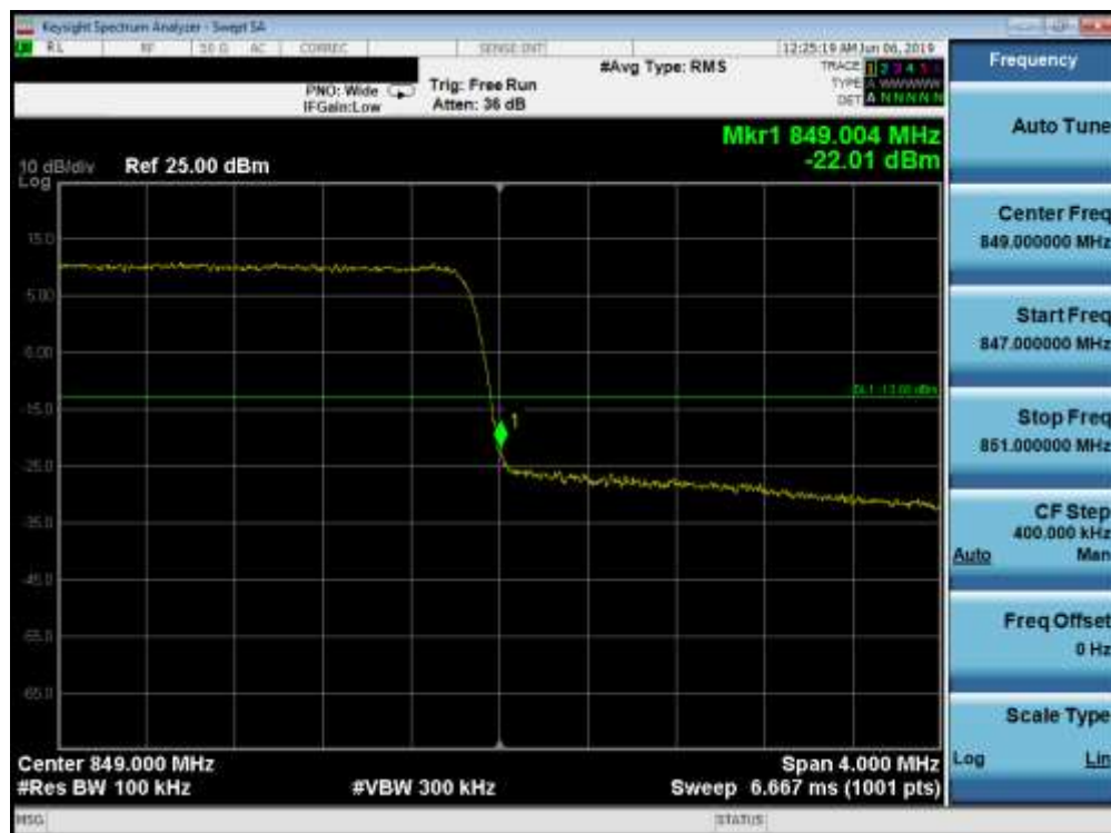
Plot 7-122. Upper Band Edge Plot (Band 5 - 3.0MHz QPSK - Full RB Configuration)
