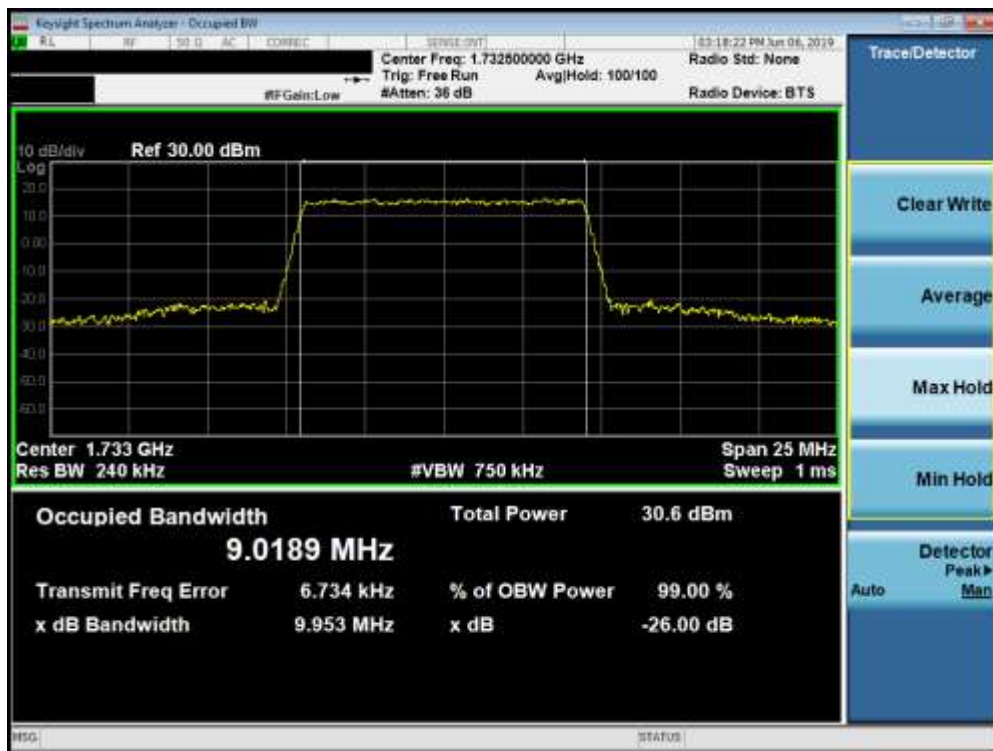
Plot 7-27. Occupied Bandwidth Plot (Band 66/4 - 10.0MHz QPSK - Full RB Configuration)
