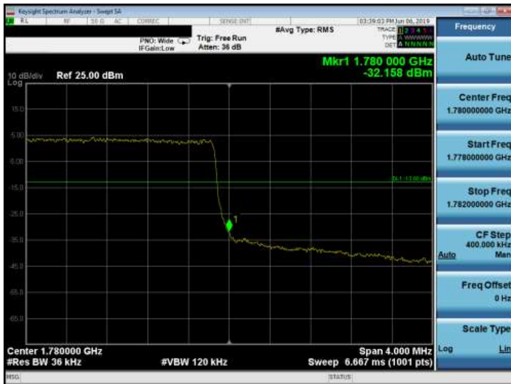
Plot 7-137. Upper Band Edge Plot (Band 66 - 3.0MHz QPSK - Full RB Configuration)
