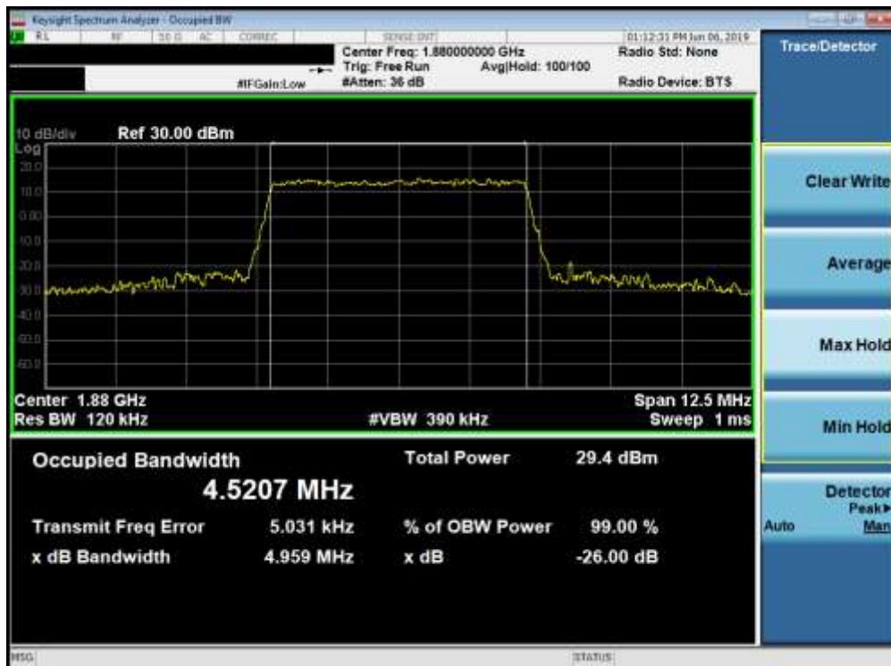
Plot 7-38. Occupied Bandwidth Plot (Band 2 - 5.0MHz 16-QAM - Full RB Configuration)
