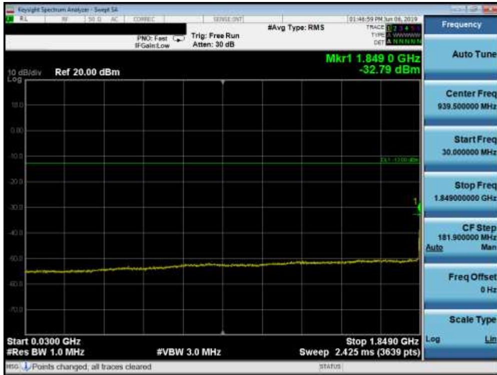
Plot 7-83. Conducted Spurious Plot (Band 2 - 20.0MHz QPSK - RB Size 1, RB Offset 0 - Low Channel)
