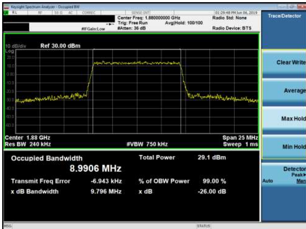
Plot 7-40. Occupied Bandwidth Plot (Band 2 - 10.0MHz 16-QAM - Full RB Configuration)
