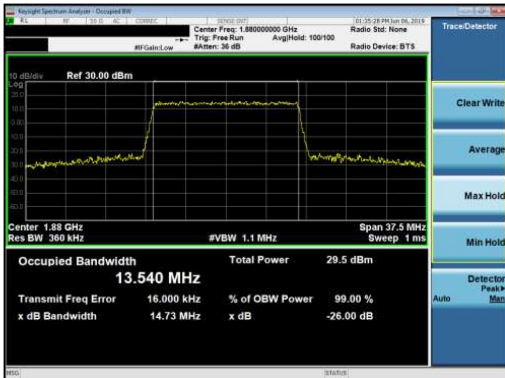
Plot 7-42. Occupied Bandwidth Plot (Band 2 - 15.0MHz 16-QAM - Full RB Configuration)
