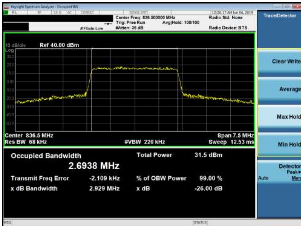
Plot 7-16. Occupied Bandwidth Plot (Band 5 - 3.0MHz 16-QAM - Full RB Configuration)
