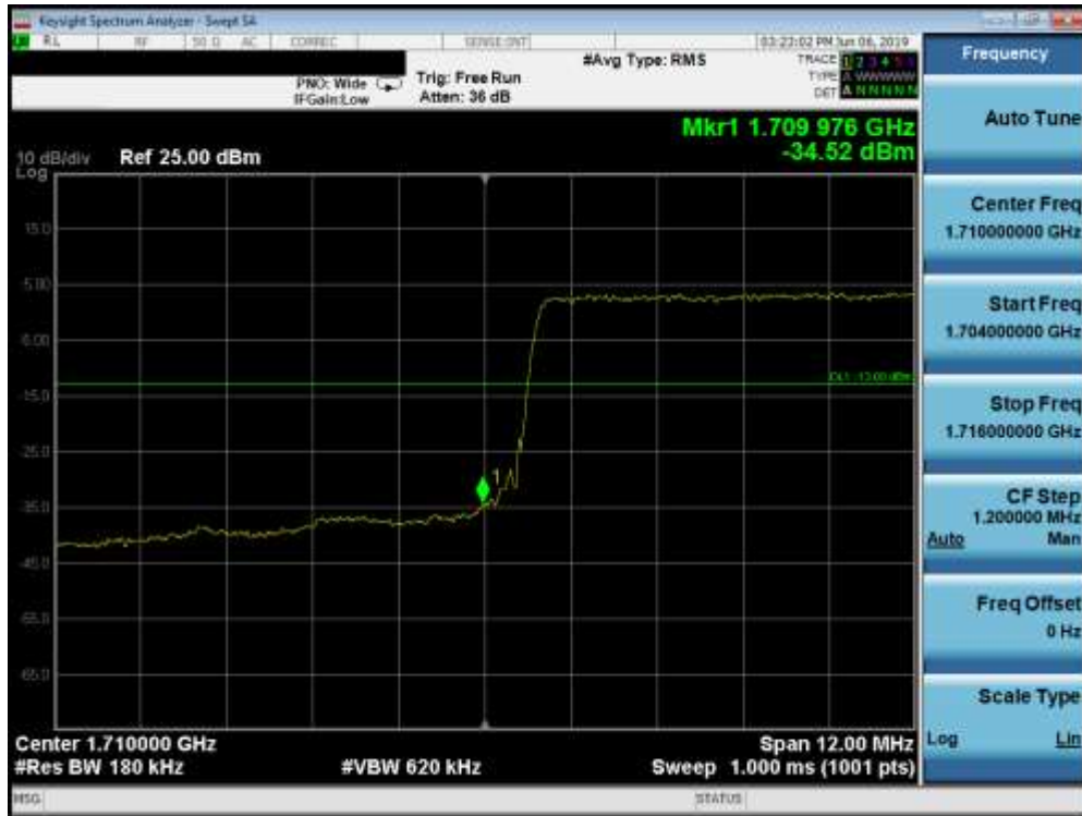
Plot 7-151. Lower Band Edge Plot (Band 66/4 - 15.0MHz QPSK - Full RB Configuration)
