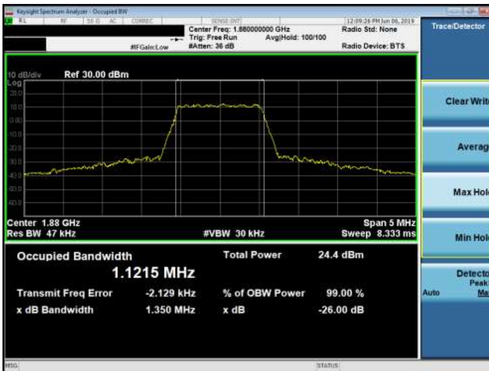
Plot 7-34. Occupied Bandwidth Plot (Band 2 - 1.4MHz 16-QAM - Full RB Configuration)
