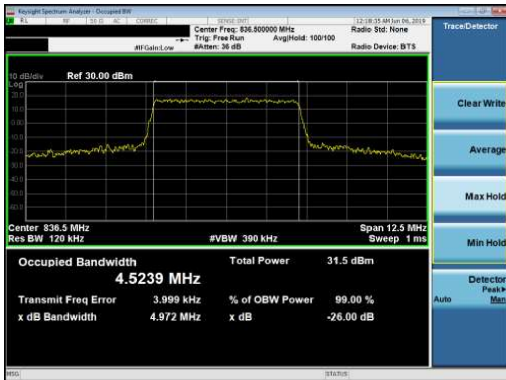
Plot 7-18. Occupied Bandwidth Plot (Band 5 - 5.0MHz 16-QAM - Full RB Configuration)
