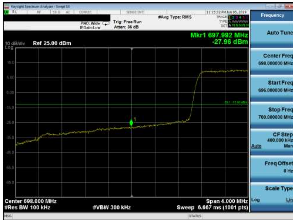
Plot 7-103. Lower Band Edge Plot (Band 12 - 3.0MHz QPSK - Full RB Configuration)
