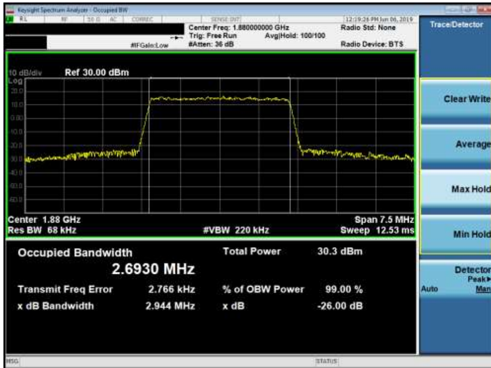
Plot 7-35. Occupied Bandwidth Plot (Band 2 - 3.0MHz QPSK - Full RB Configuration)
