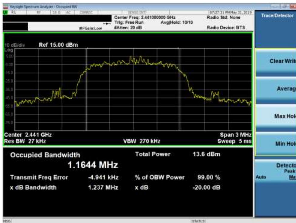
Plot 7-5. 20dB Bandwidth Plot (Bluetooth, 2Mbps – Ch. 39)
