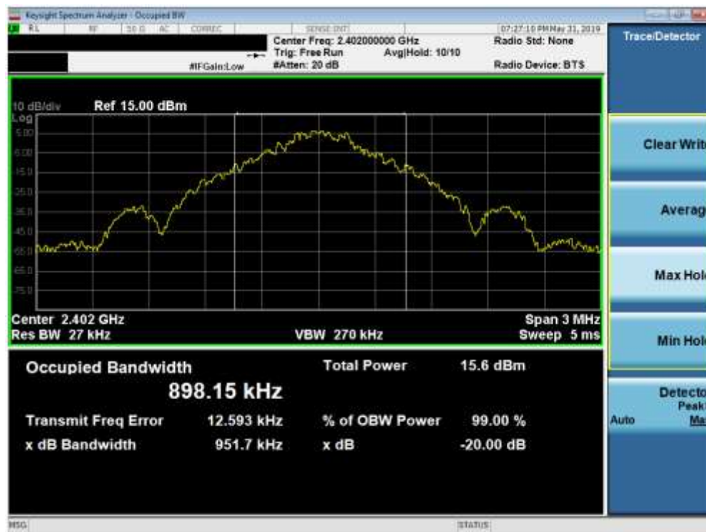
Plot 7-1. 20dB Bandwidth Plot (Bluetooth, 1Mbps – Ch. 0)
