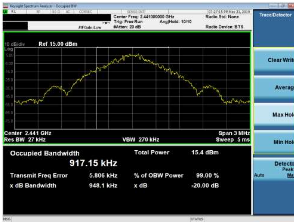
Plot 7-2. 20dB Bandwidth Plot (Bluetooth, 1Mbps – Ch. 39)
