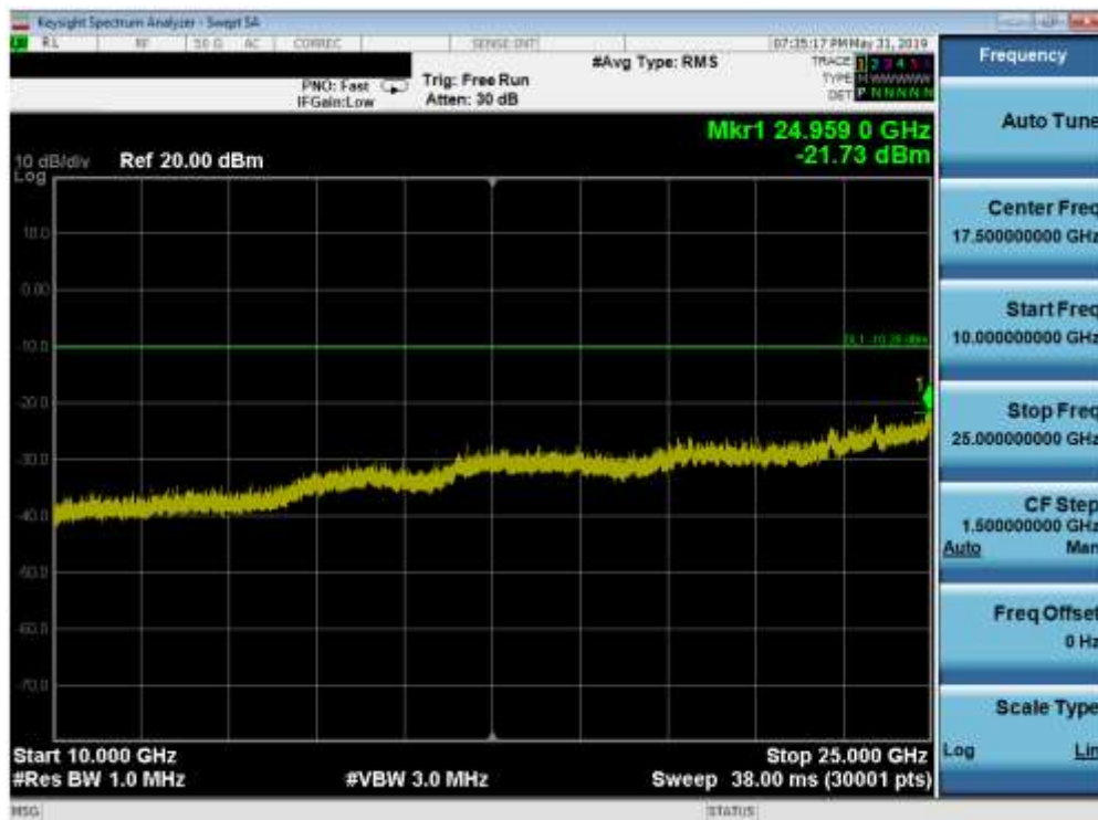
Plot 7-41. Conducted Spurious Plot (Bluetooth, 1Mbps – Ch. 78)
