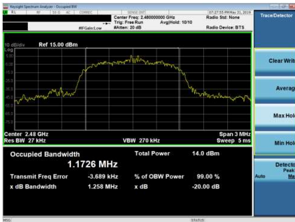
Plot 7-9. 20dB Bandwidth Plot (Bluetooth, 3Mbps – Ch. 78)
