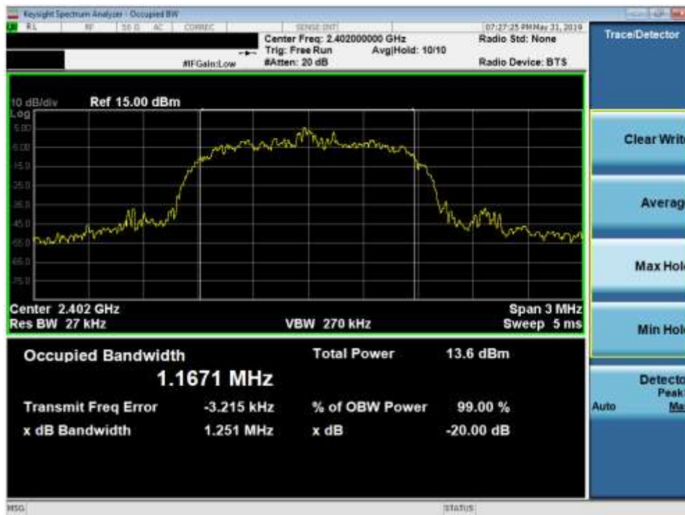
Plot 7-4. 20dB Bandwidth Plot (Bluetooth, 2Mbps – Ch. 0)
