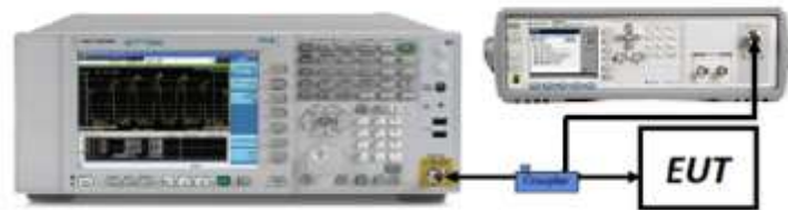
Figure 7-1. Test Instrument & Measurement Setup
