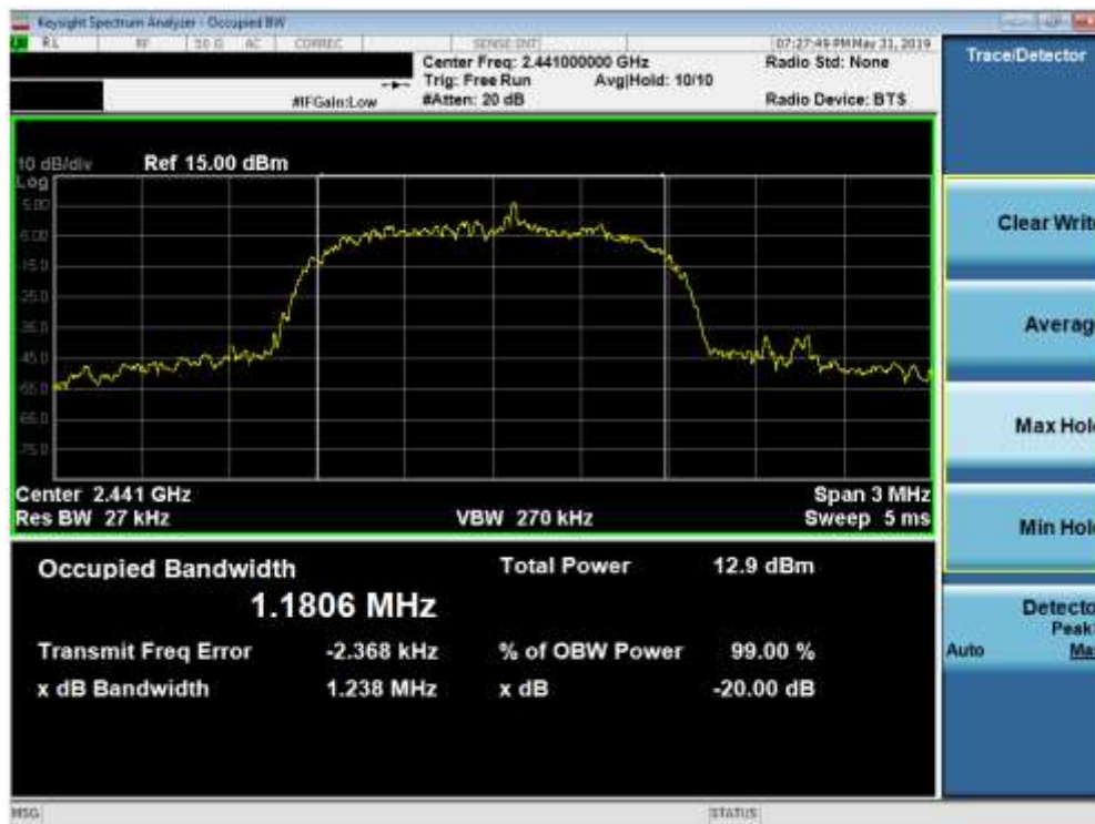
Plot 7-8. 20dB Bandwidth Plot (Bluetooth, 3Mbps – Ch. 39)
