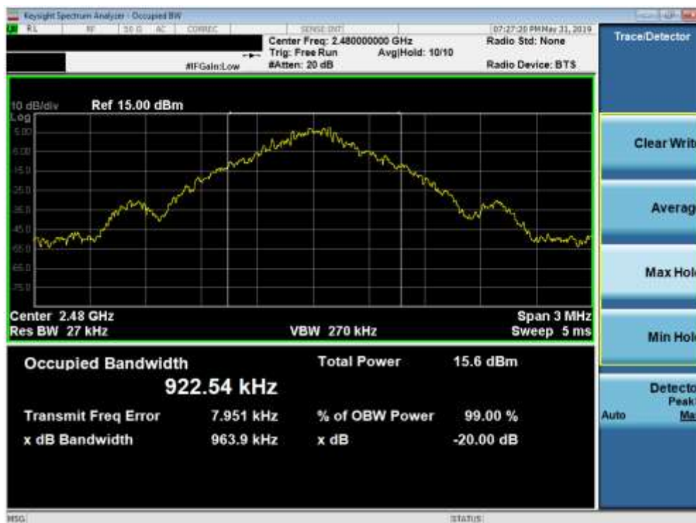
Plot 7-3. 20dB Bandwidth Plot (Bluetooth, 1Mbps – Ch. 78)
