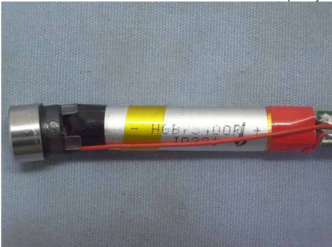
Figure 8 Internal View (Battery View)
