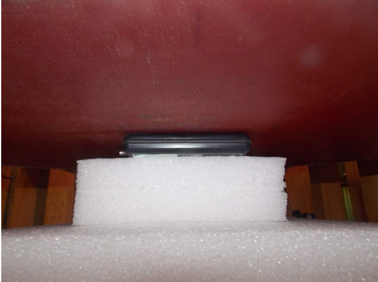
Test Position Back 0 mm Gap
