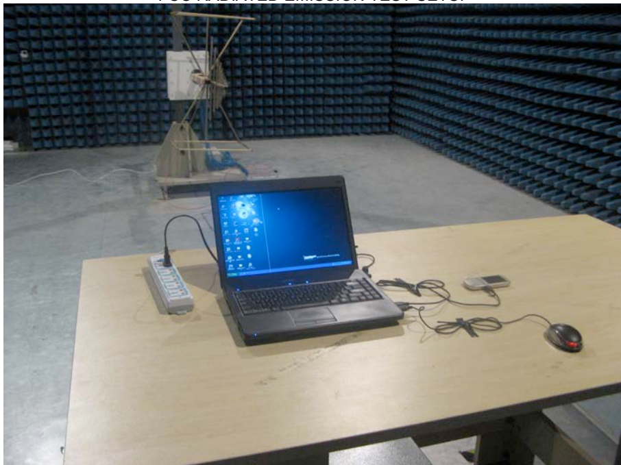
FCC RADIATED EMISSION TEST SETUP
