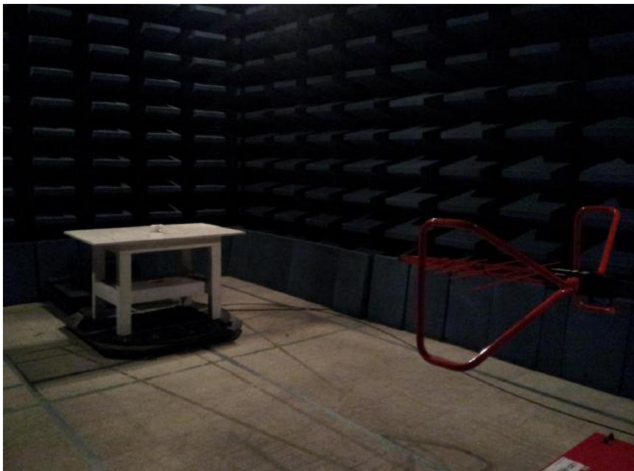
Radiated Emissions Test-Setup 30MHz-1GHz
