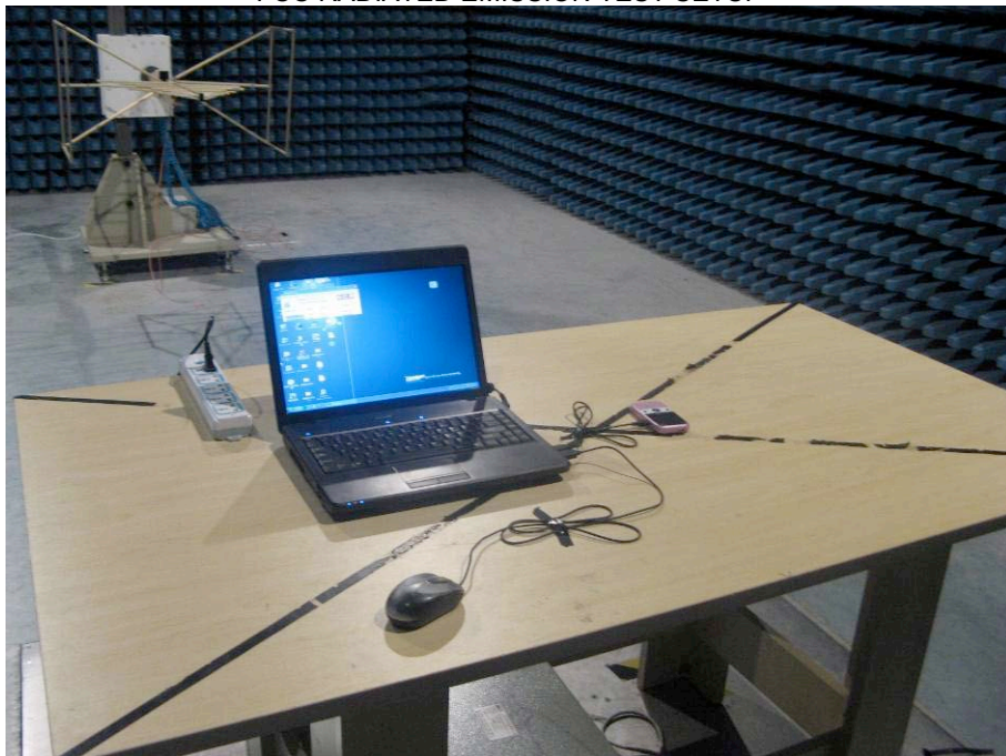
FCC RADIATED EMISSION TEST SETUP
