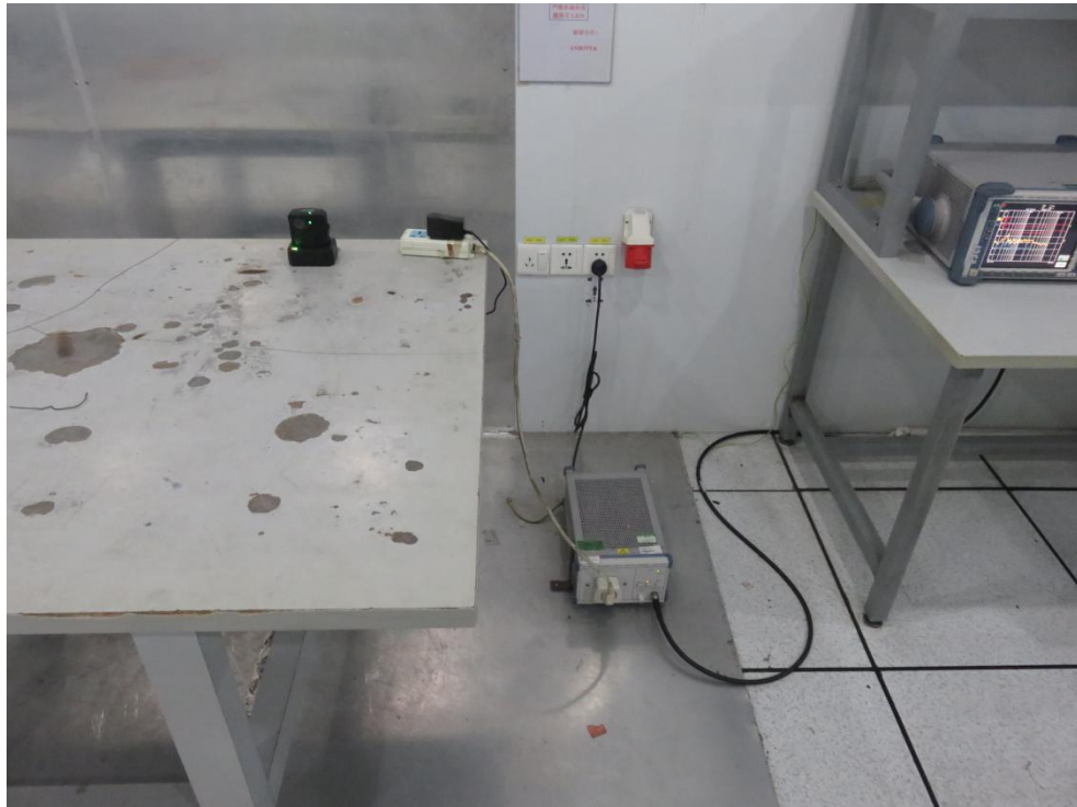
Photo of Conducted Emission Measurement
