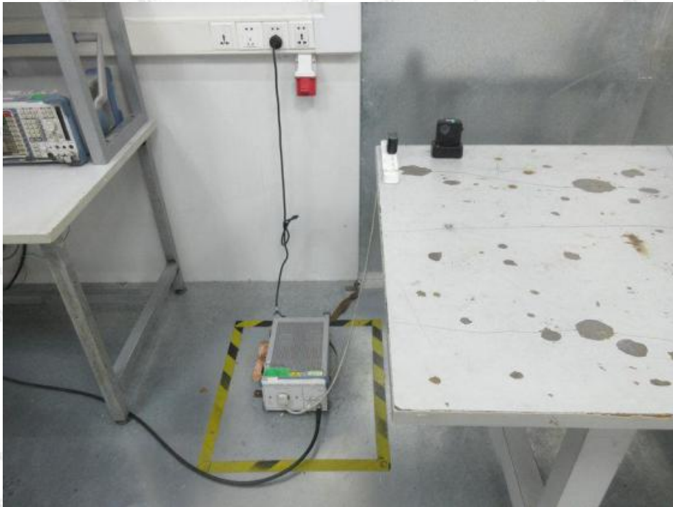
Photo of Power Line Conducted Emission Test
