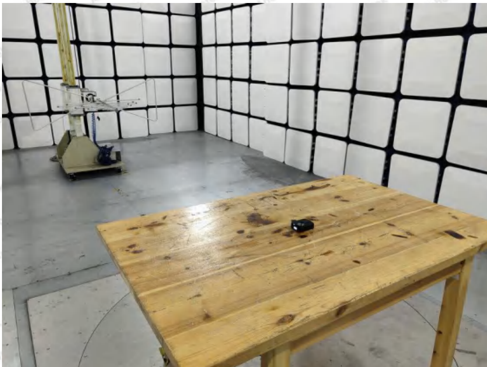
Photo of Radiation Emission Test
