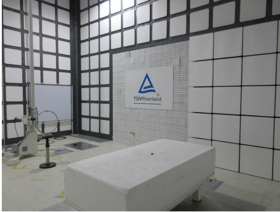
Photograph 4: Test Setup for Spurious Emissions (Back View 2)
