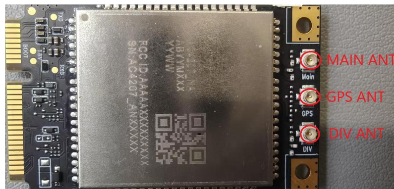
Figure 5-1 Module Antenna Schematic Diagram
