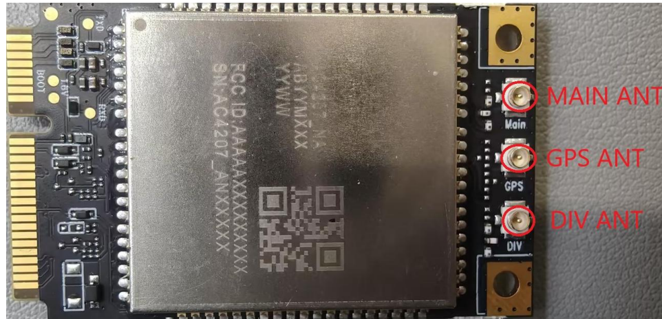
Figure 3-12 Module Antenna Schematic Diagram
