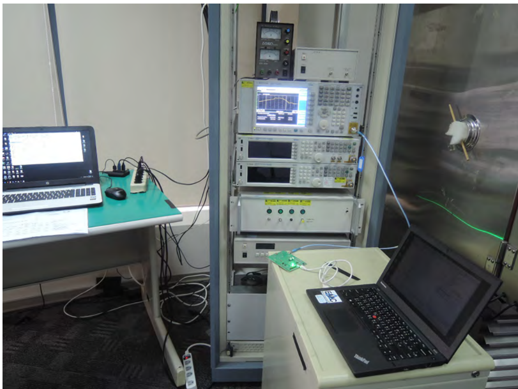
Photograph 5: Set-up for Conducted testing
