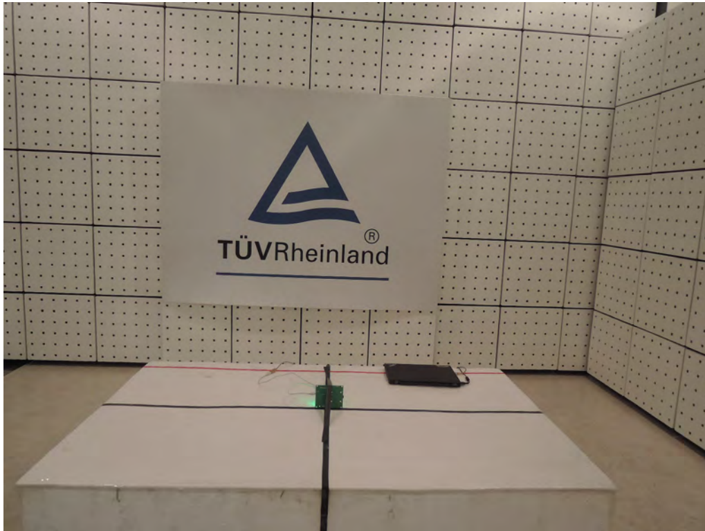
Photograph 1: Set-up for Spurious Emissions (Front View)
