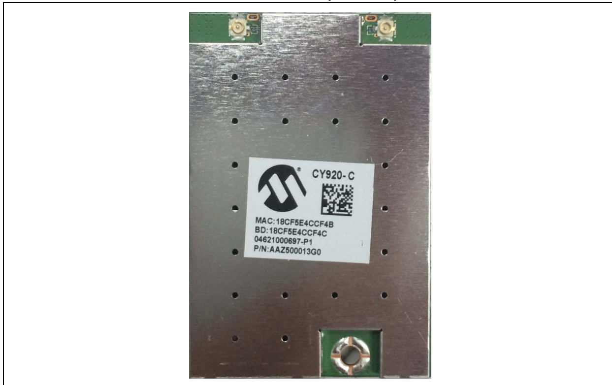
FIGURE 2-3: CY920 BOARD WITH RF SHIELD (TOP VIEW)
