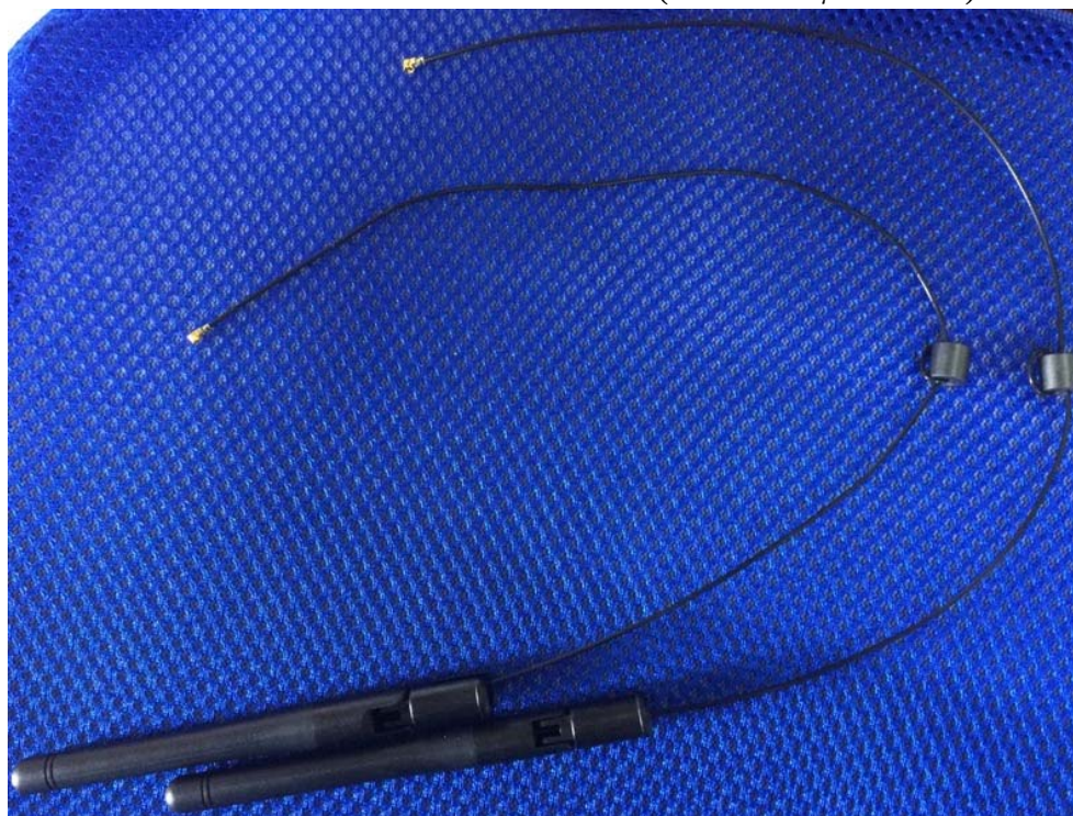
(40) EUT Photo - WALSIN / RFDPA870933IMLB302 (ferrite core \varnothing 8.0*4mm)
