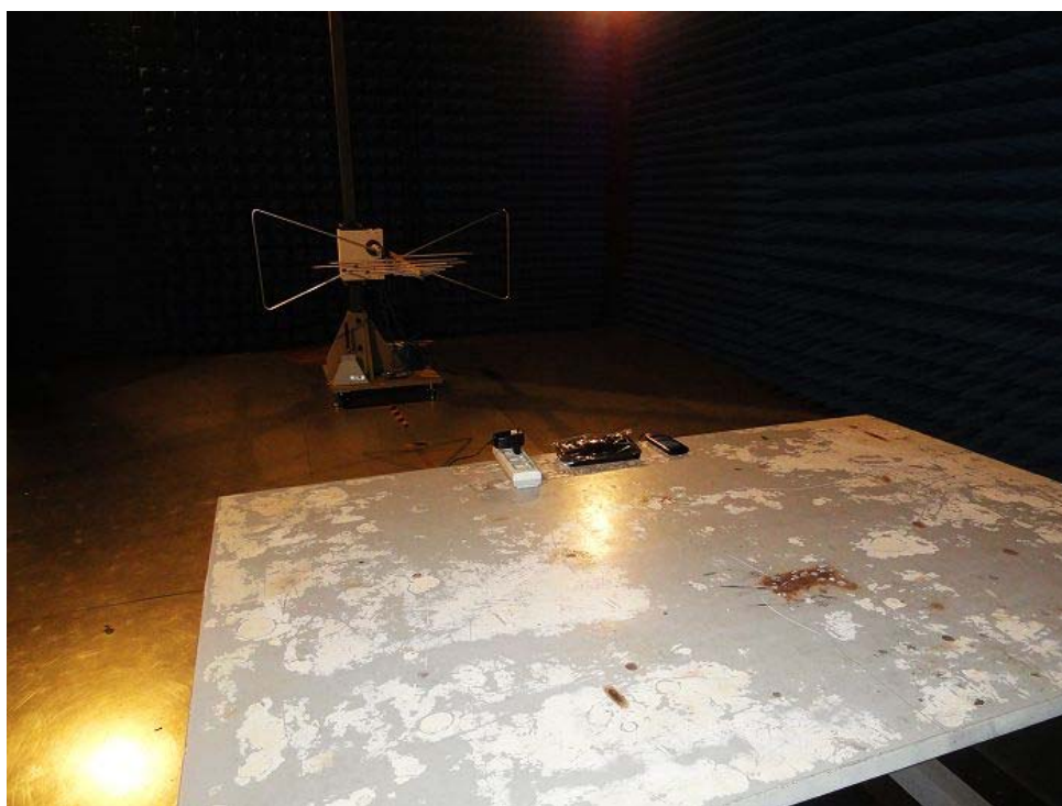
Radiated emission test view
