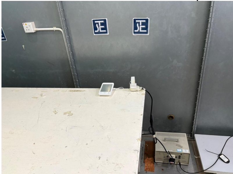
Measurement of Conducted Emission Test Set Up
